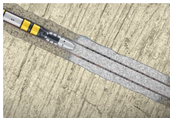
f) Cementing process
