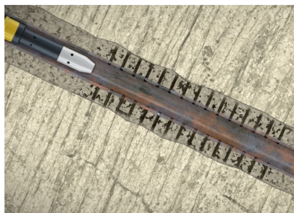
b) Perforated plugging zone
