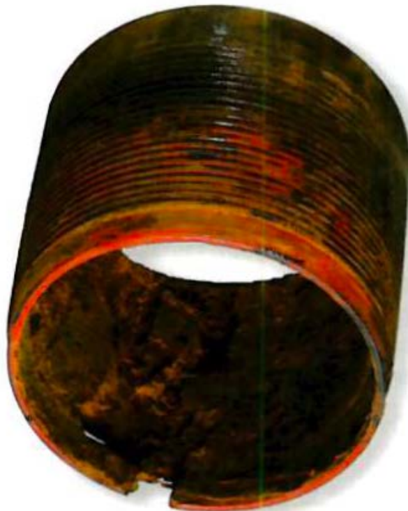
Figure 2.7: Corroded water injecting carbon steel tubing (Bellarby, 2009).
