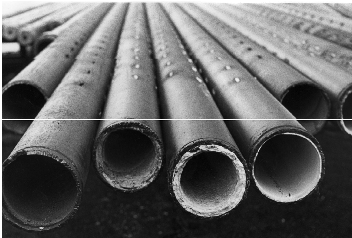
Figure 2.8: Calcite Scaling Inside a Slotted Liner in Krafla KJ-19 (Fridriksson & Thórhallsson).
