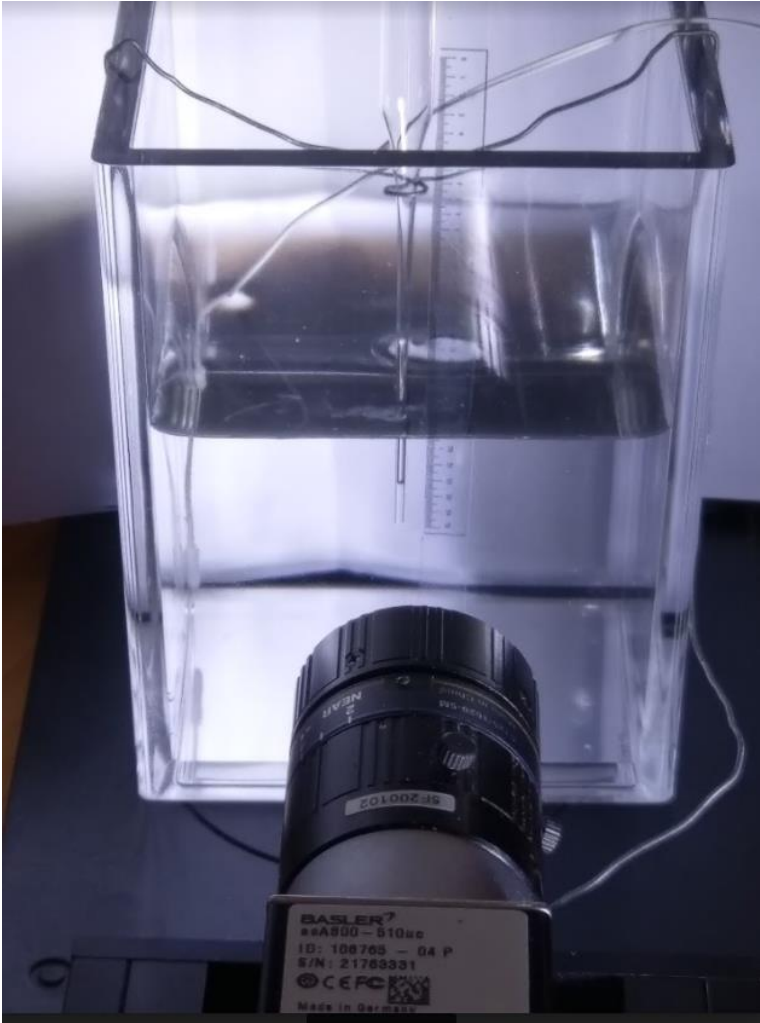
Figure 45: Camera recording images from the tip of capillary tube
