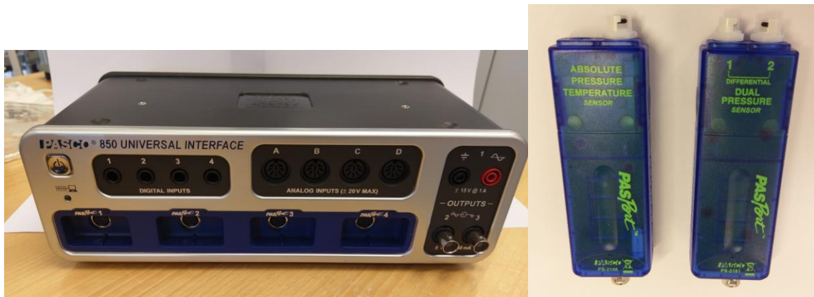
Figure 16: PASCO Universal Interface (left) and two sensors (right).
