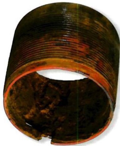
Figure 14. Corrosion on water injection tubing [8]
