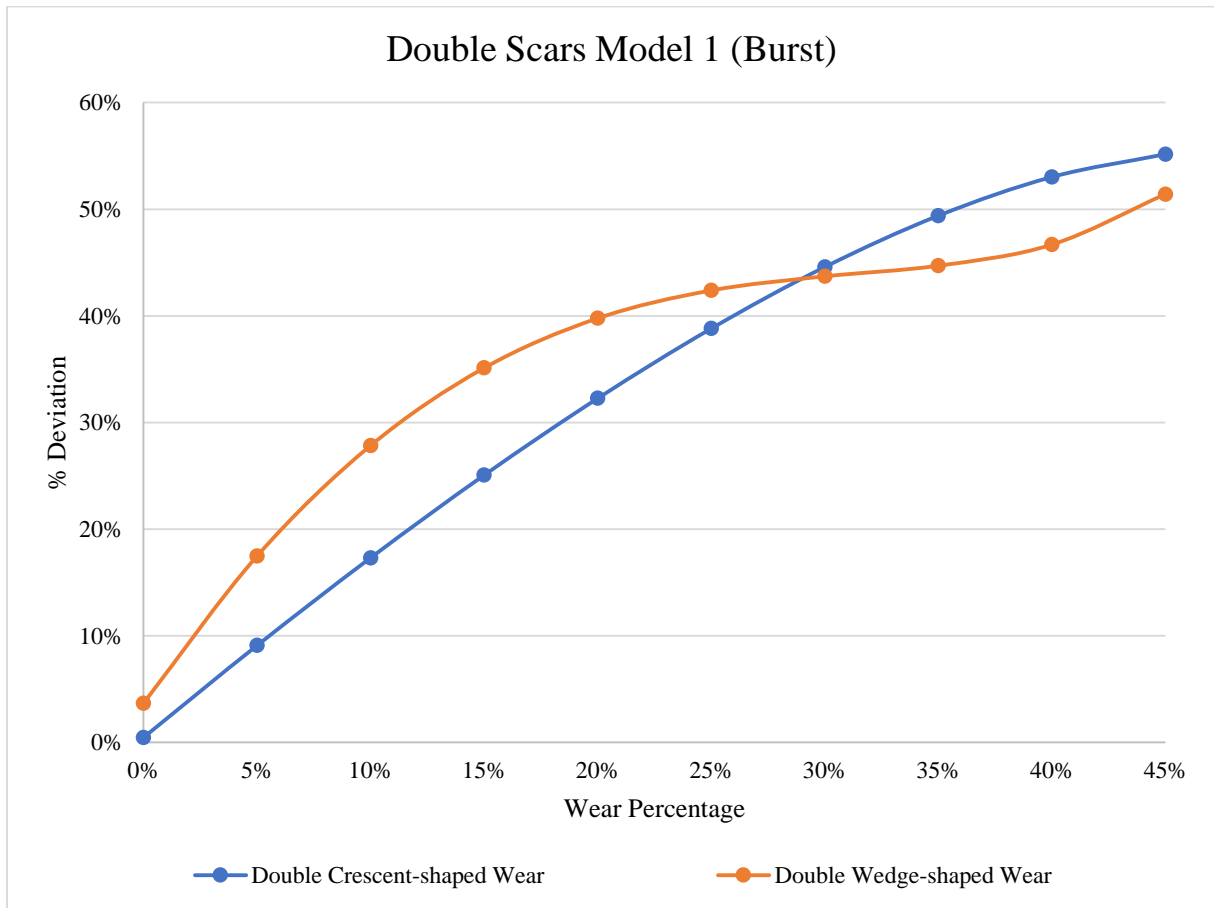
Figure 90. Deviation Percentage between API Burst/Barlow model and FEM simulation results for different double scars scenarios (model 1)
