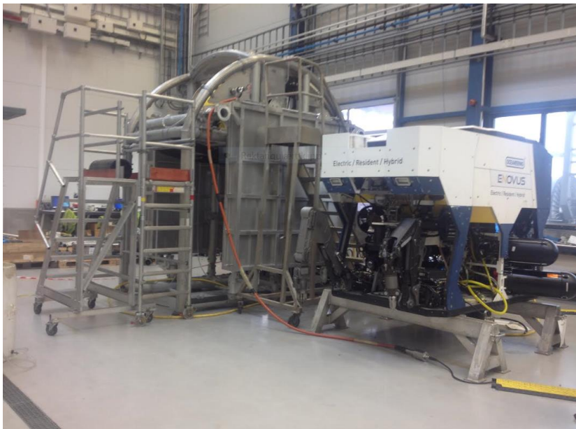
Figure 18 – Oceaneering eROV manufacturing plant Stavanger, Norway. eROV under construction. The ROV cage is seen on the left in the picture with large battery packs to be installed on the sidewalls of the ROV cage. (picture Bråten, Erik, 18.05.2017)
