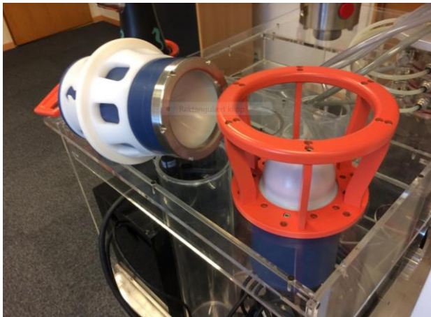
Figure 25 – Blue Logic Subsea USB receptacle from visit 29.09.17 (Photo, Bråten, Erik 2017)
