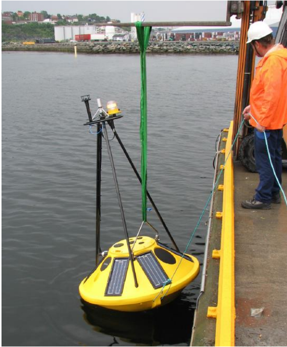
Figure 26 – Fugro Seawatch Midi 185 buoy (Fugro.com, 2017) (Source; Fugro.com (2017) Official website (online) Available at: https://www.fugro.com/about-fugro/our-expertise/technology/seawatch-metocean-buoys-and-sensors (Accessed 29.09.2017))
