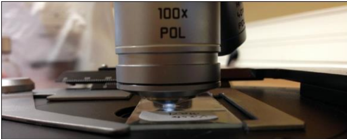
Figure 16: Oil drop between the objective and the smear slide to increase the numerical aperture and the resolution.
