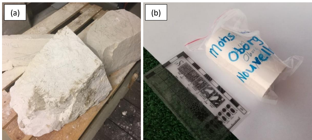
Figure 9: (a) Big blocks of chalk samples that were collected originally from Kansas before being cored in University of Stavanger. (b) An example of prepared cylindrical core samples; Mons, limit Obourg Nouvelles; the sample has a length of approximately 8.5cm.
