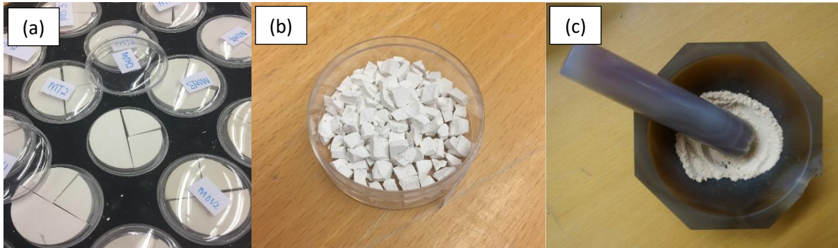
Figure 12: (a) Sections of chalk samples are quartered where each quarter is used for palaeontology study and stored into transparent containers. (b) Samples snipped into pellet form and ready to be used in SSA measurement and analysis. (c) Samples being powdered using mortar to avoid the destruction of minerals.
