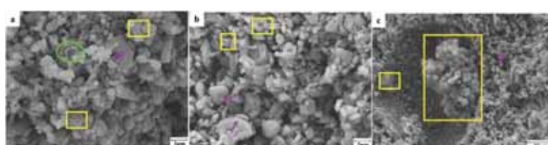
Fig. 3. (A) Clay-minerals, preserved opal-CT and coccolithophores in the Na130 (slice 7); (b) SEM-micrograph of NaCl-flooded LNa130 (slice 2). Partly preserved opal-CT (yellow square) are widespread. (c) Large cluster of opal-CT found inside foraminifera shells in LNa130 (slice 6). Yellow square: opal-CT; pink arrow: coccoliths; green circle: clay minerals. (For interpretation of the references to colour in this figure legend, the reader is referred to the Web version of this article.)
