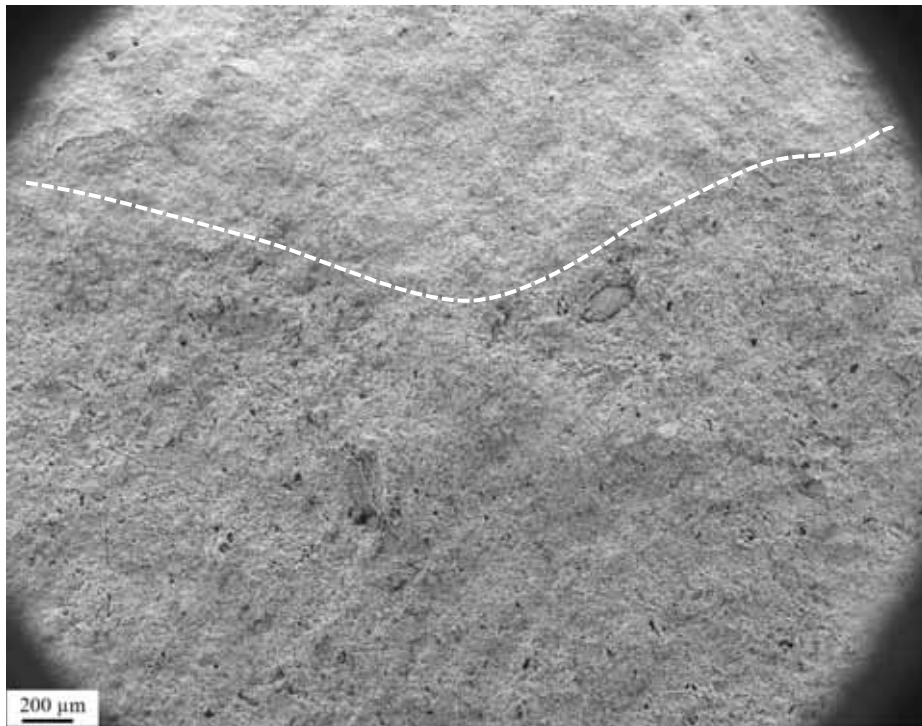
Figure 18: FEG-SEM micrograph of the transition-zone in the LTT with increased porosity, below the white dashed line, compared to the area still dominated by the original calcite mineralogy to the top of the image.
