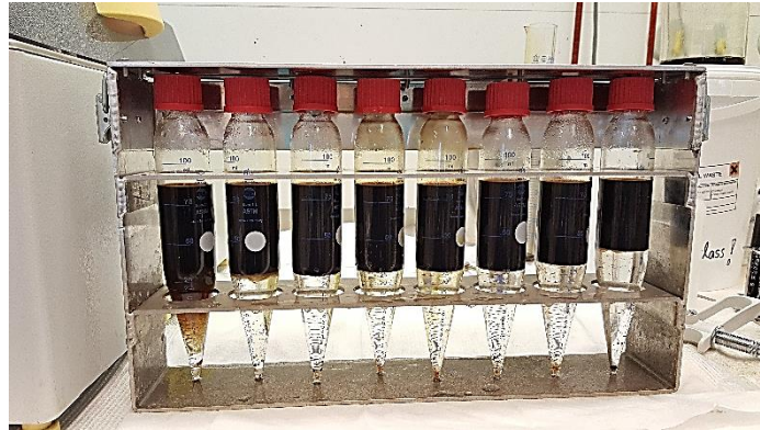
Figure 3. 4 Torpedo flasks in rack used for demulsifier testing.
