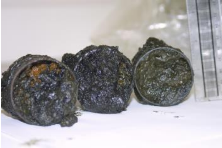
Figure 3.5: Biofilms in pipes (Hoffmann and Spark, 2012).
