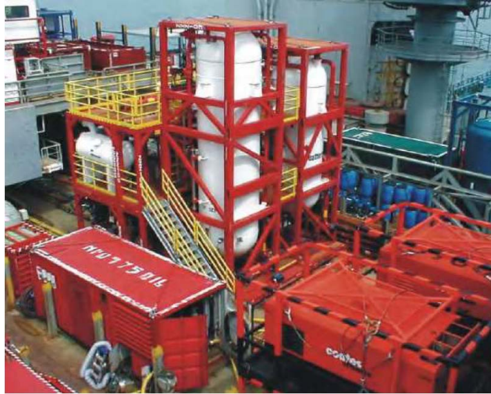
Figure 2.15: MPD Multiphase Separation System (Sveinall, 2010)
