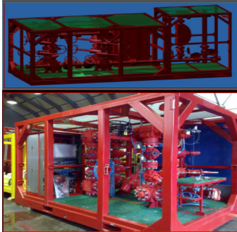
Fig 26: Automatic Choke Skid [20]
