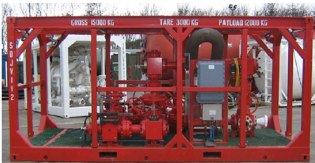
Fig 32: Combined Choke Manifold, Coriolis Flow meter and control system [19]
