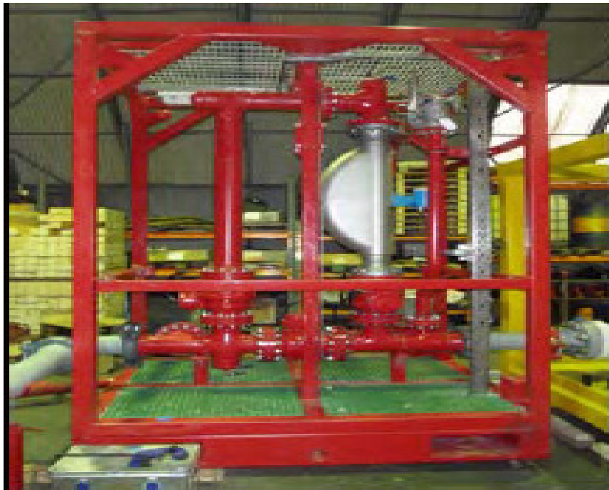
Fig 27: A Metering Skid [20]
