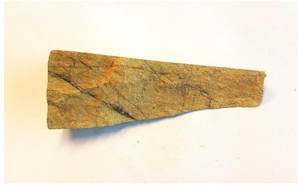
Figure 34 Chalk core photographs of microfractures.
