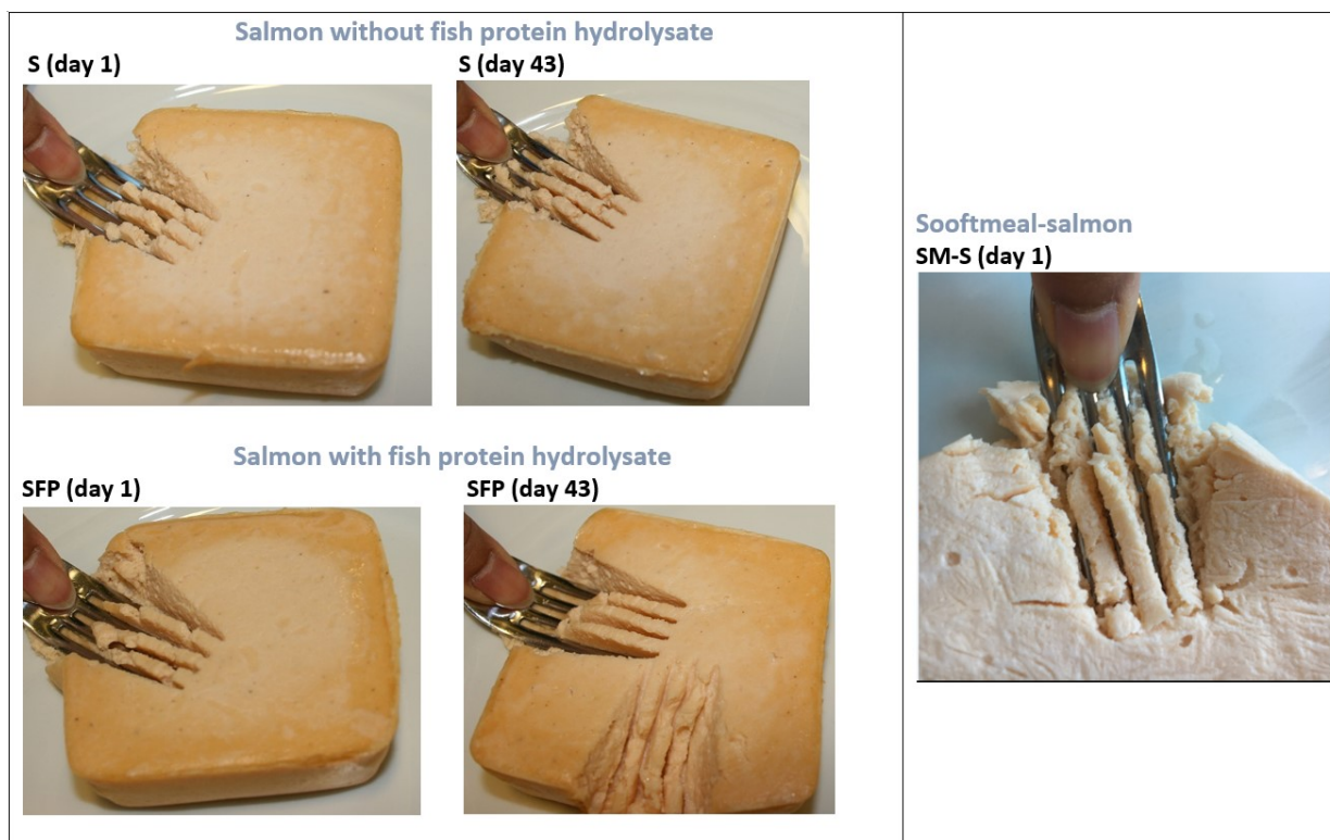
Figure 4.7 IDDSI Fork test performed on salmon without protein hydrolysate(S) and with hydrolysate(SFP) on day 1 and day 43. Fork test on reference sample softmeal-salmon (SM-S) on day 1.
