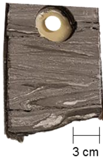
Figure 11: Convoluted bedding in heterolithics (facies D2) taken from core 6507/3-9S (2876-2877 m depth).
