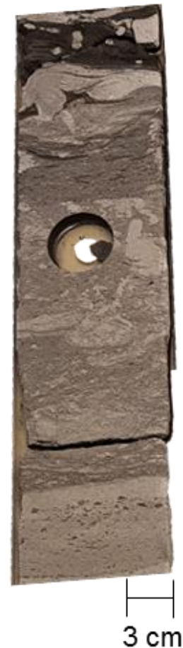
Figure 10: Core 6507/3-9S. Heterolithics (facies D2) with sand injectites, mud clasts and water escape structures (2881-2882 m depth).
