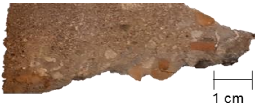
Figure 7: Breccia (facies A) from core 6507/2-2 with 3 mm to 1 cm large angular grains (3290 m depth).
