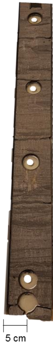
Figure 9: Graded and laminated sandstone facies (facies C). The picture is taken from core 6507/3-9S (2861-2862 m depth).
