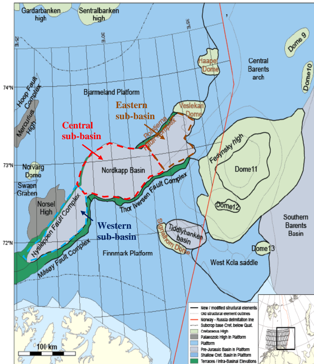
Figure 10. Structural elements of the Southern Barents Sea region. Modified after Mattingdal et al., 2015
