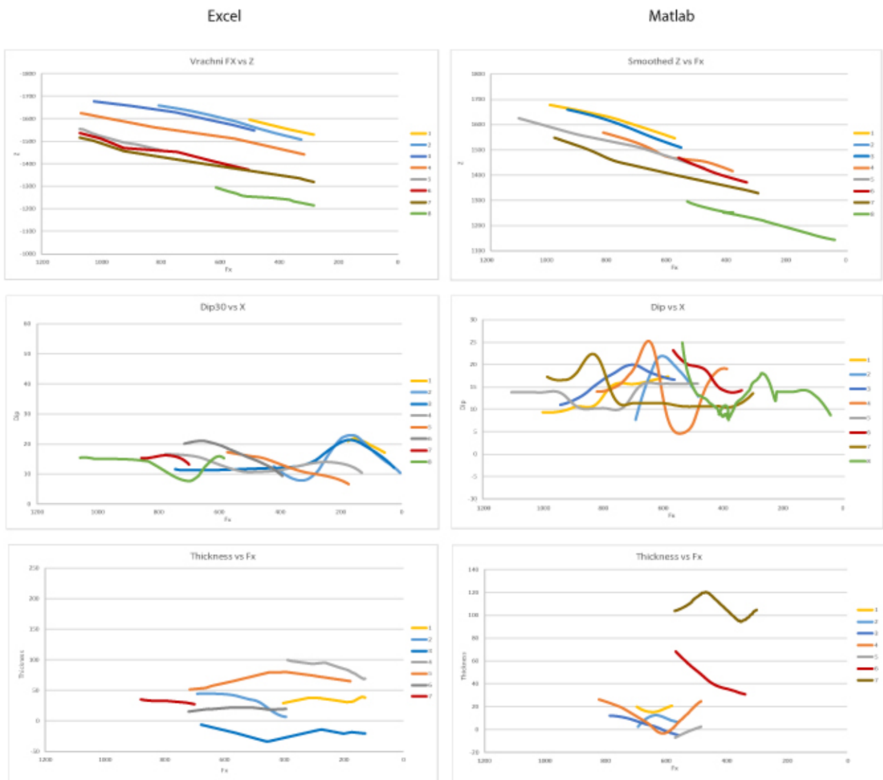
Figure 3.26: Structural analysis of Vrachni outcrop displaying bedding line, dip and thickness plots achieved applying two approaches utilizing Excel and Matlab software.
