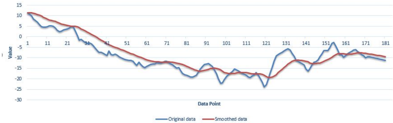
Figure 3.11: Illustration of exponential smoothing effect on one bedding line. The original line data is displayed in blue, while the smoothed data is displayed in red. Exponential smoothing evens out fluctuations in the original data using data by applying smoothing along the bedding line.
