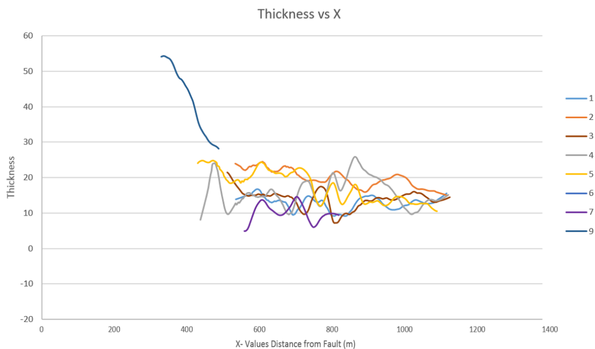
Figure 4.6: Thickness variation plot illustrating thickness value fluctuations of the Lapanagoi outcrop.
