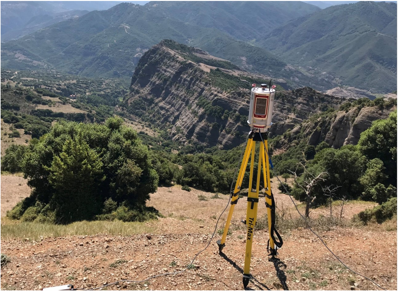
Figure 3.2: The image of LiDAR RIEGL VZ-6000 3D terrestrial laser scanner acquiring data of Lapanagoi outcrop.
