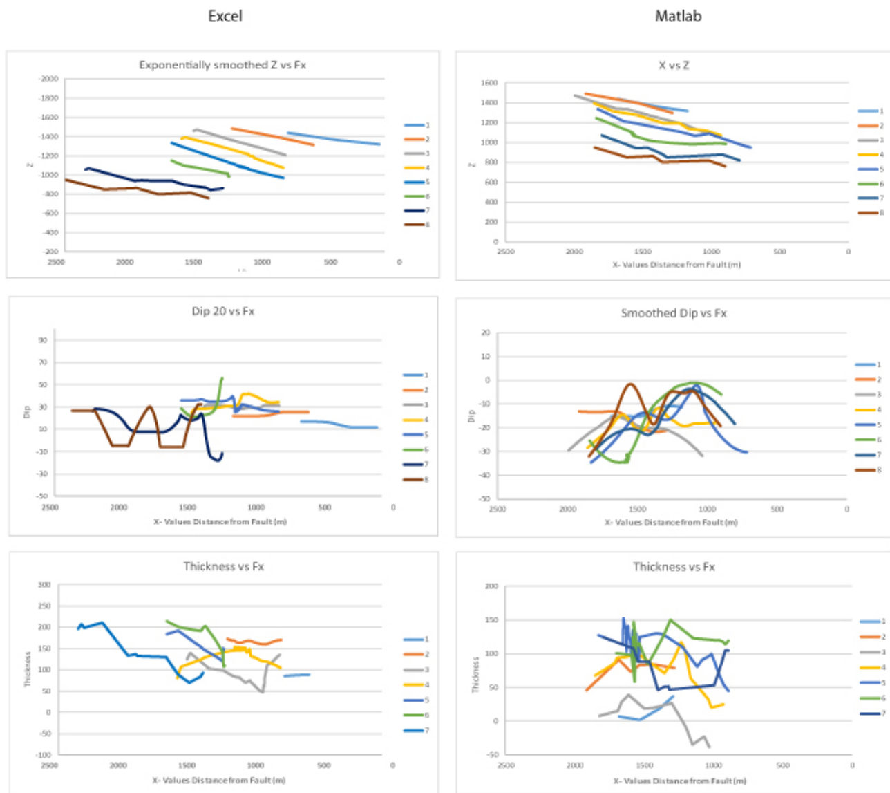
Figure 3.25: Structural analysis of Roghi outcrop displaying bedding line, dip and thickness plots achieved applying two approaches utilizing Excel and Matlab software.
