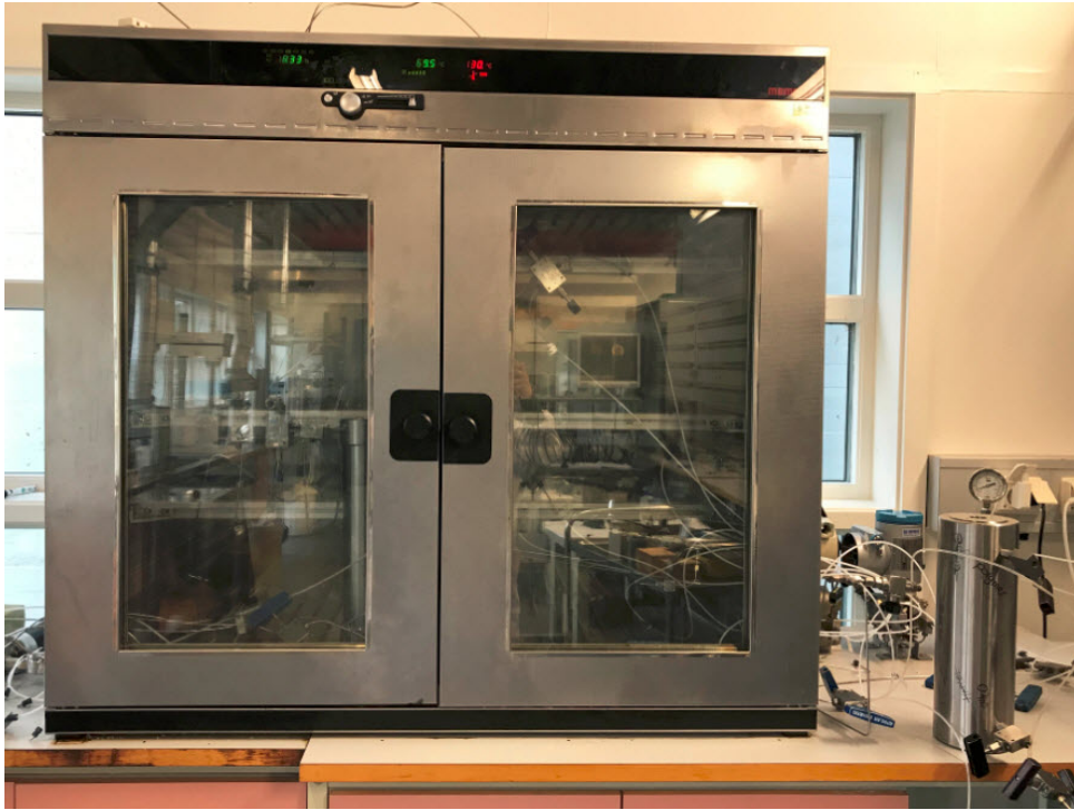
Figure 3.4: Oven containing the core holder at 70 °C.
