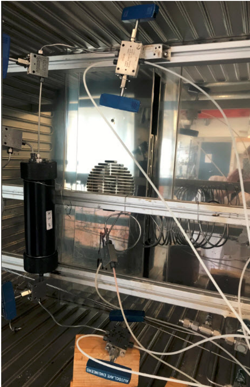
Figure 3.8: Vertical core (part 3) mounted in the oven. The coil is shown on the right side of the core.
