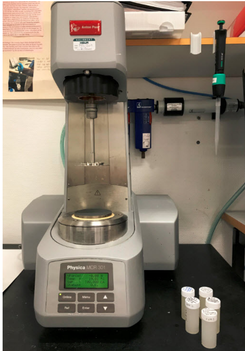
Figure 3.2: Anton Paar physica MCR 301 rheometer with cone-plate.
