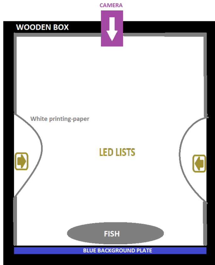
FIGURE 3.4: The design of the fish-photobox prototype. This is a vertical cut. The dark grey color represents the normal white printing-paper. The camera, shown as purple, was attached in a hole from above with Field Of View pointing down. Yellow, represents the LED lists, attached 17cm above the ground plate, pointing inwards. Also, the figure shows how the fish is placed relative to camera, on a blue background.
