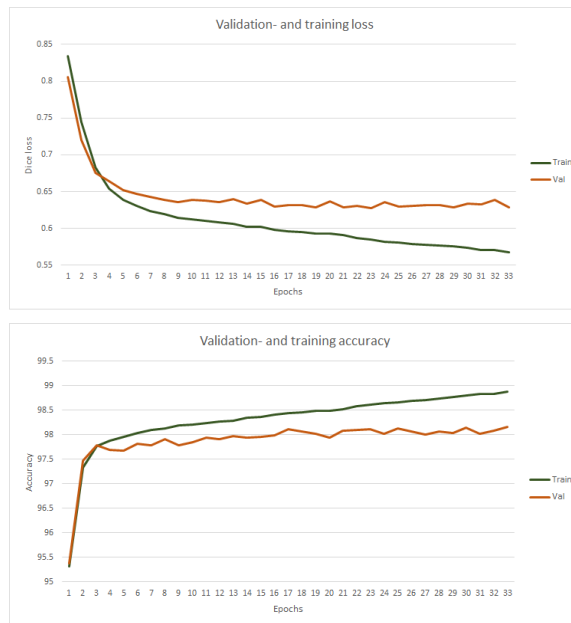
Figure 5.9: Validation- and training graphs with the use of ADAM and Dice loss, learning rate=0.0001
