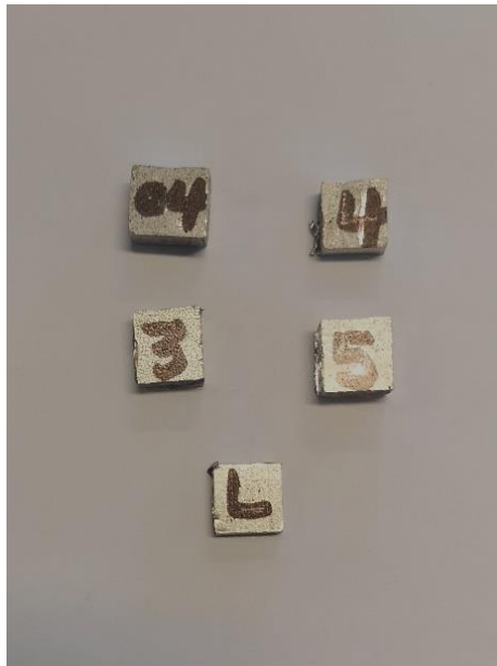
Figure 18: Samples cut for SEM-analysis
