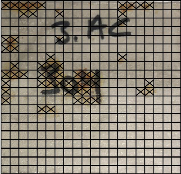
Figure 27: 20x20 grid illustrated on sample 3.AC 304
