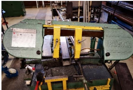
Figure 10: Rusch horizontal metal cutting band saw Figure 11: Pilous ARG 220 plus band saw
