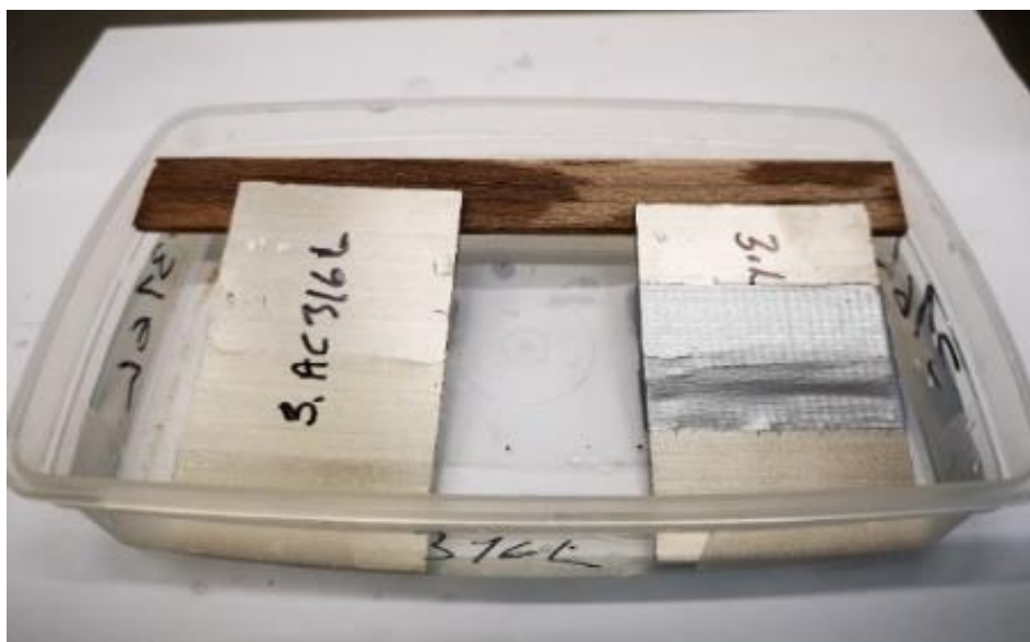
Figure 15: Samples ready for general and localized corrosion testing
