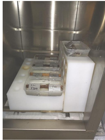
Figure 17: Samples inside the heating cabinet
