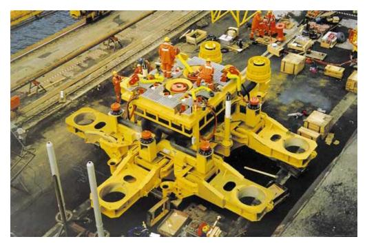
Figure 19. Five slot subsea template [42].
