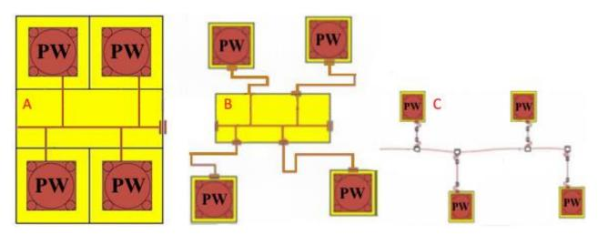
Figure 20. A - Subsea well template, B - Clustered satellite wells, C - Satellite wells. PW means production well.
