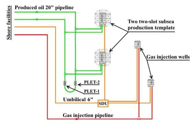
Figure 28. Proposed subsea production system layout.
