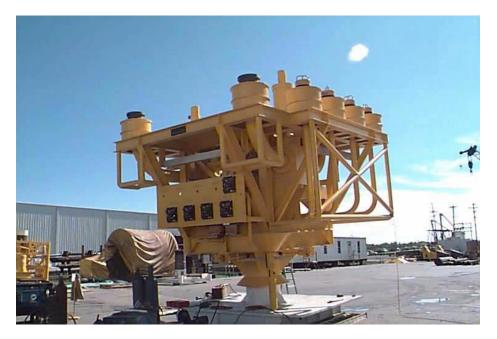
Figure 16. Example of a 4-Well Subsea Manifold [42].
