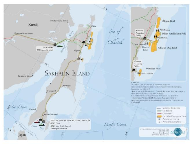
Figure 29. Sakhalin pipeline system [48].
