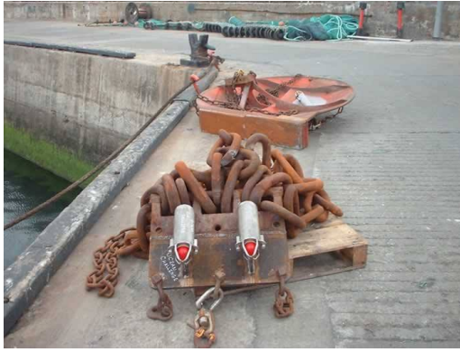
(a) An example of a primitive type of clump weight, which is just a chain link (Photo credit: Notus Electronics)
