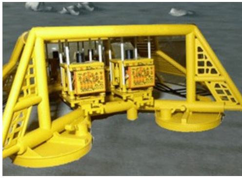
Figure 2.3: A typical subsea template with wellheads and the steel protective cover over it (Photo credit: FishSafe)
