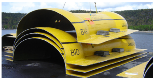
Figure 2.4: A typical subsea GRP cover (Photo credit: Stangeland Glassfiberprodukter AS)
