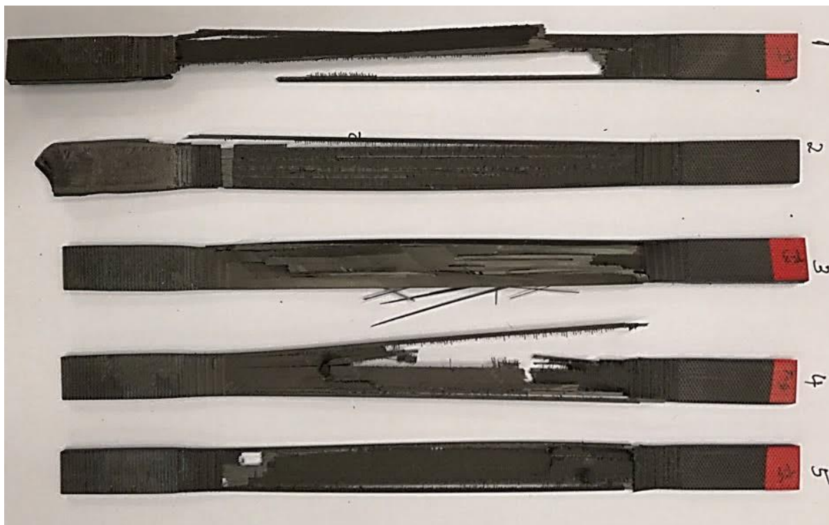
b) Failed unidirectional tensile samples S1, S2, S3, S4, S5 from top to bottom.
