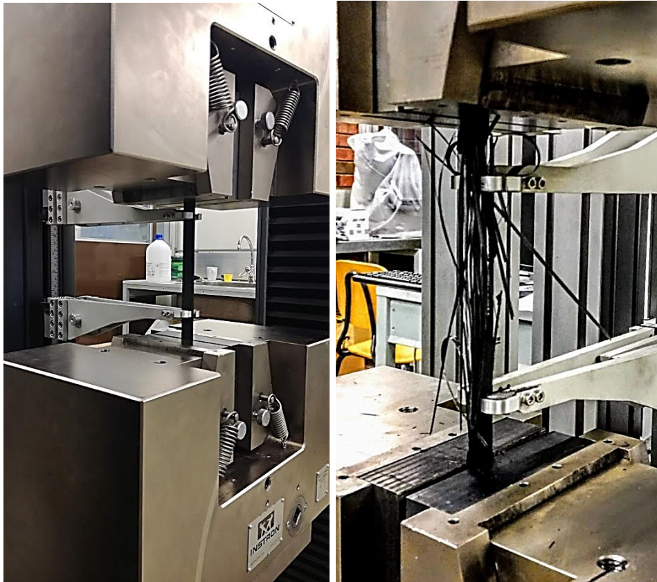
Figure 4-2. (a).Tensile Testing Instron universal testing machine setup , (b) explosive failure of S3
