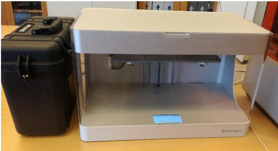
Figure 2-1. Markforged® Mark-Two 3D printer for composites and airtight box
