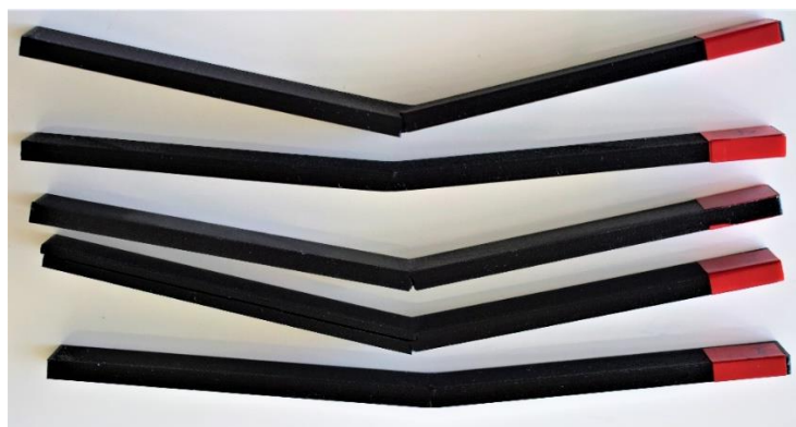
Figure 4-5. Failed sample of flexural test
