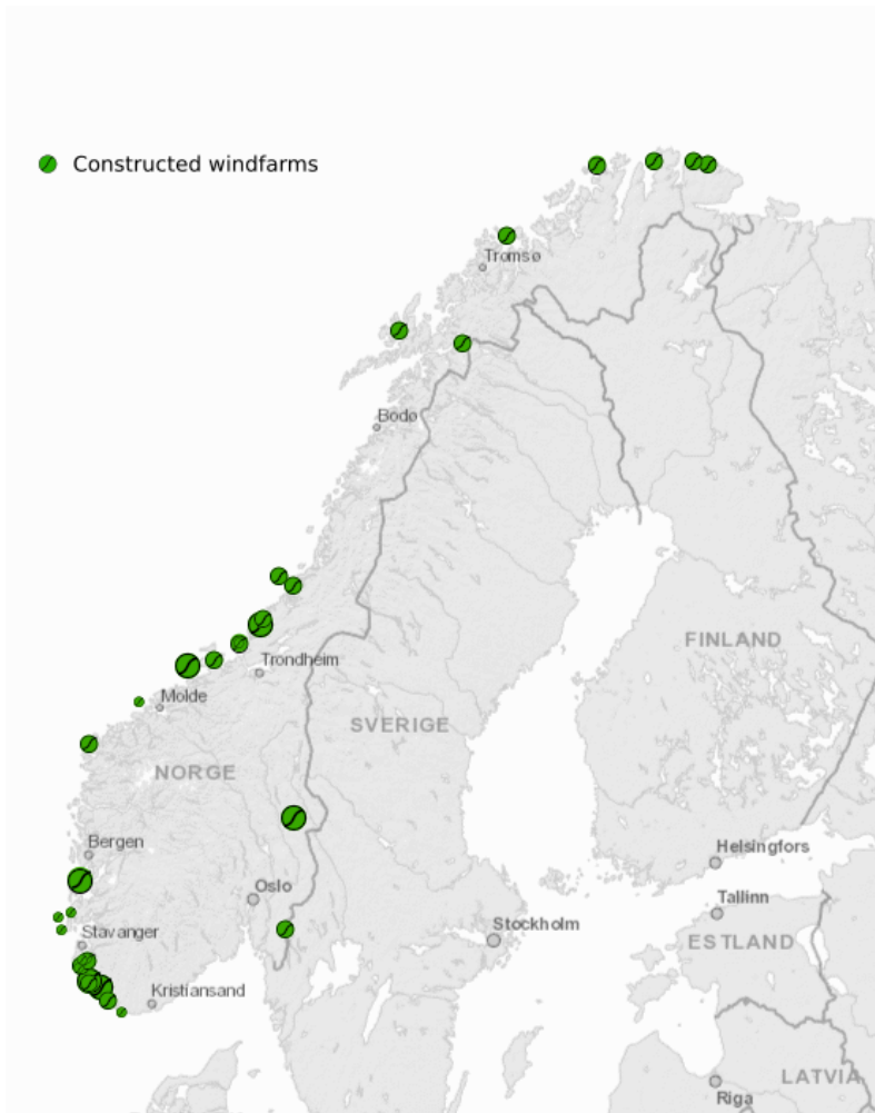
Figure 1.2: Constructed wind-farms in Norway, the size of the markers differentiate between the power output of the wind-farms, ranging from 10, 10-100 and >100 MW
