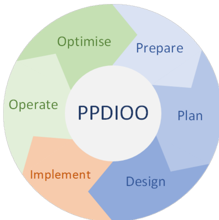
Figure 16: Prepare, Plan, Design, Implement, Operate, and Optimize (PPDIOO) Lifecycle Framework. Source:[21]
