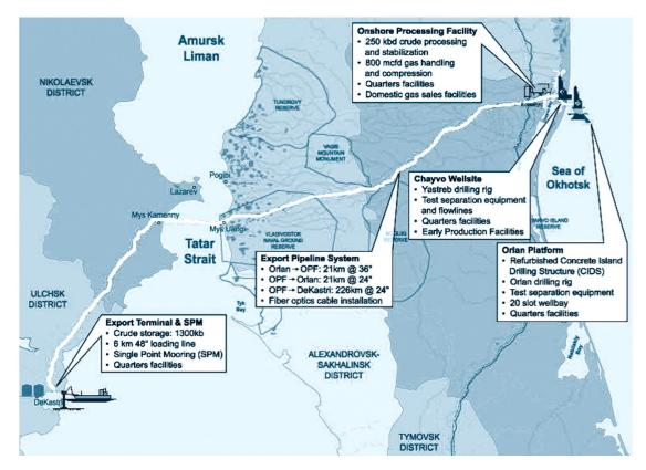
Figure 4 Overview of the Sakhalin-1 project including the Chayvo OPF, Chayvo Wellsite, Orlan Platform, Export Pipeline System crossing the Tatar Strait, and the Export Terminal and SPM Offloading Facilities at De Kastri (Joep Athmer and Teus Gijzel, 2006)
