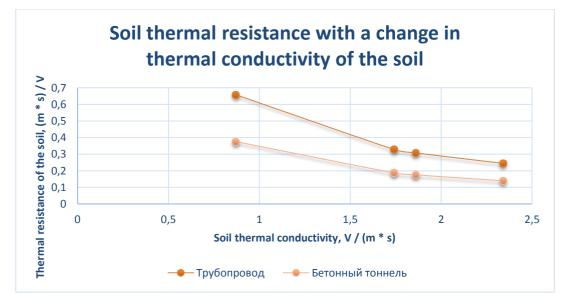
Figure 31 Soil thermal resistance vs soil thermal conductivity
