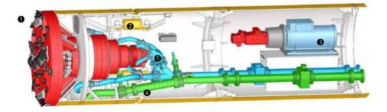
• Cutting head • Steering cylinder • Drive unit • Removal pipe • Feeding pipe
