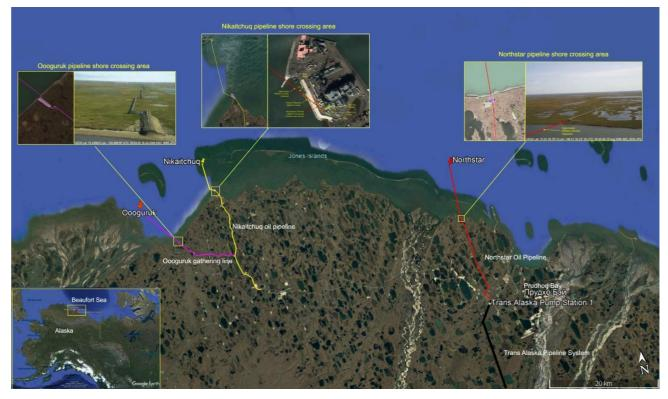
Figure 7 The Beaufort Sea Pipelines with Shore Crossing Areas (made by author with the use of Google Earth)
