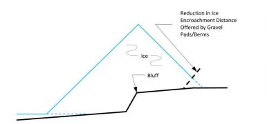
Figure 12 Shoreline Ice Encroachment (Eisler, B., 2016)
