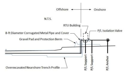
Figure 1 Northstar Shore Crossing Scheme (Eisler, B. 2016)
