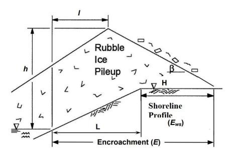
Figure 11 Geometric Parameters Used in Predicting Encroachment (Coastal Frontiers, 2012)
