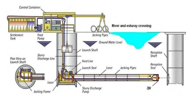
Figure 27 Scheme of Tunnel
