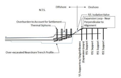
Figure 3 Ooguruk Shore Crossing Scheme (Eisler, B. 2016)
