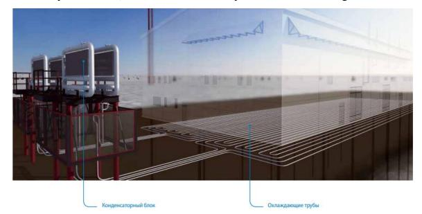
Figure 32 Horizontal tubular cooling system (NPO Fundamentstroyarkos LLC)
