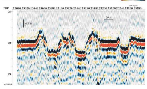
Figure 6 Ice Ridges Traces of Plowing (Mironuk, S., 2014)
