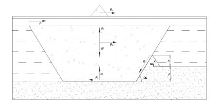
Figure 15: Force System on Ice Ridge (Duplenskiy S., 2012)
