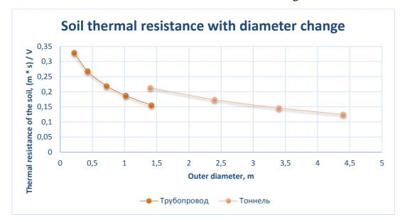
Figure 30 Soil thermal resistance vs diameter change
