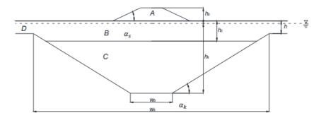
Figure 14 Cross section view of a ridge (ISO 19906)
