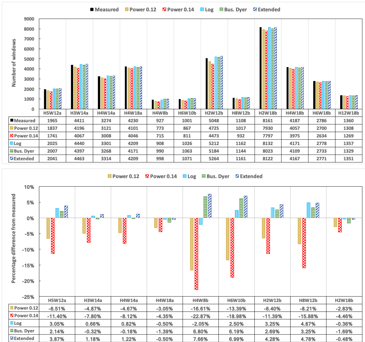
Figure 5.4: Number of available wind weather windows in measured data compared to extrapolated data from wind profile models.
