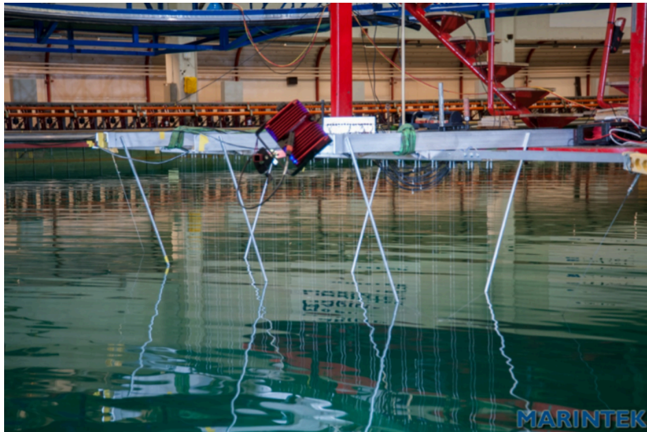
Figure 1: Wave Gauge Apparatus used for testing in the MARINTEK Ocean Laboratory
