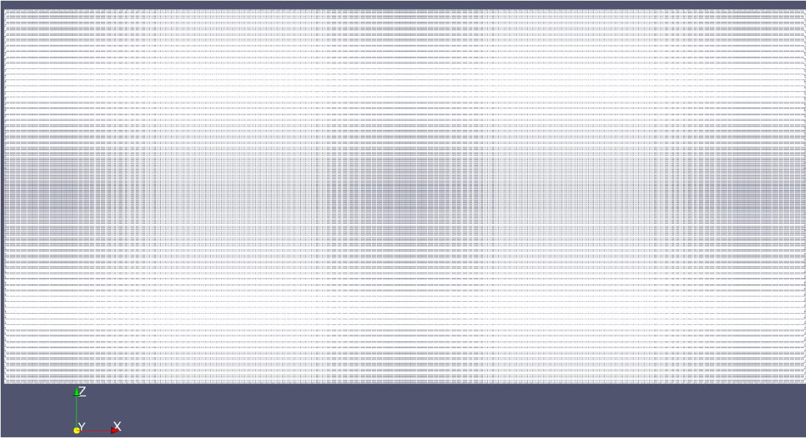
Figure 10: Full computational mesh, having dimensions of 15\text{m} \times 0.1\text{m} \times 7\text{m} , in the x, y, and z directions, constructed using the computational cells illustrated in Figure 9
