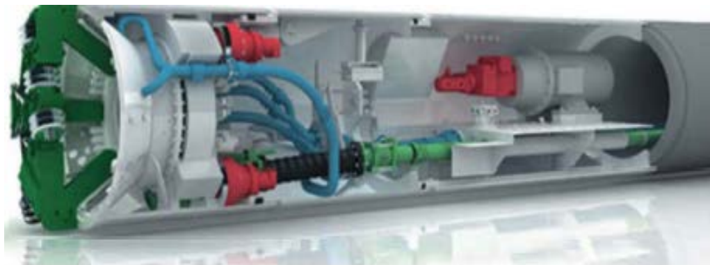
Figure 4.7. AVN1200T Herrenknecht Microtunnelling Machine [32]
