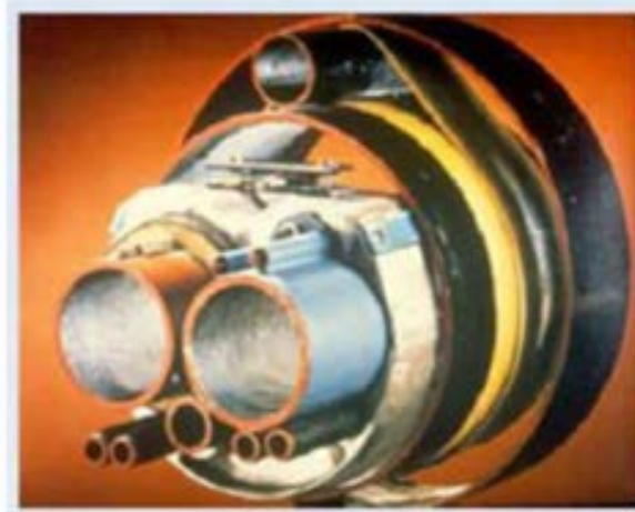
Figure 3.1. Cross-section of the Drake Project Pipeline [1]
