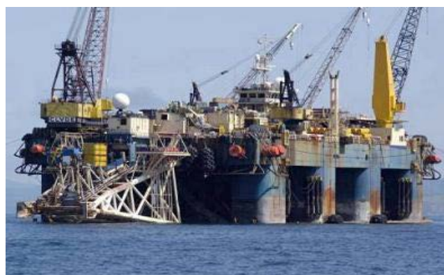
Figure 3.8. Pipe-laying Barge «Seamac» [9]
