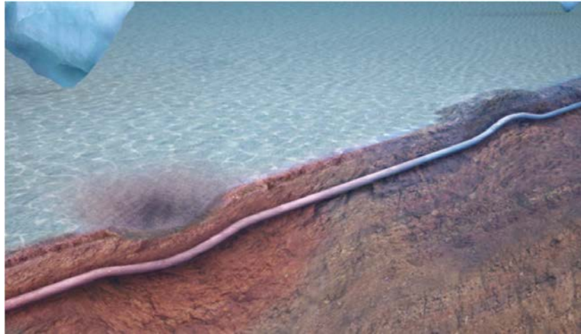
Figure 4.3. Permafrost Thawing Near the Pipeline [19]
