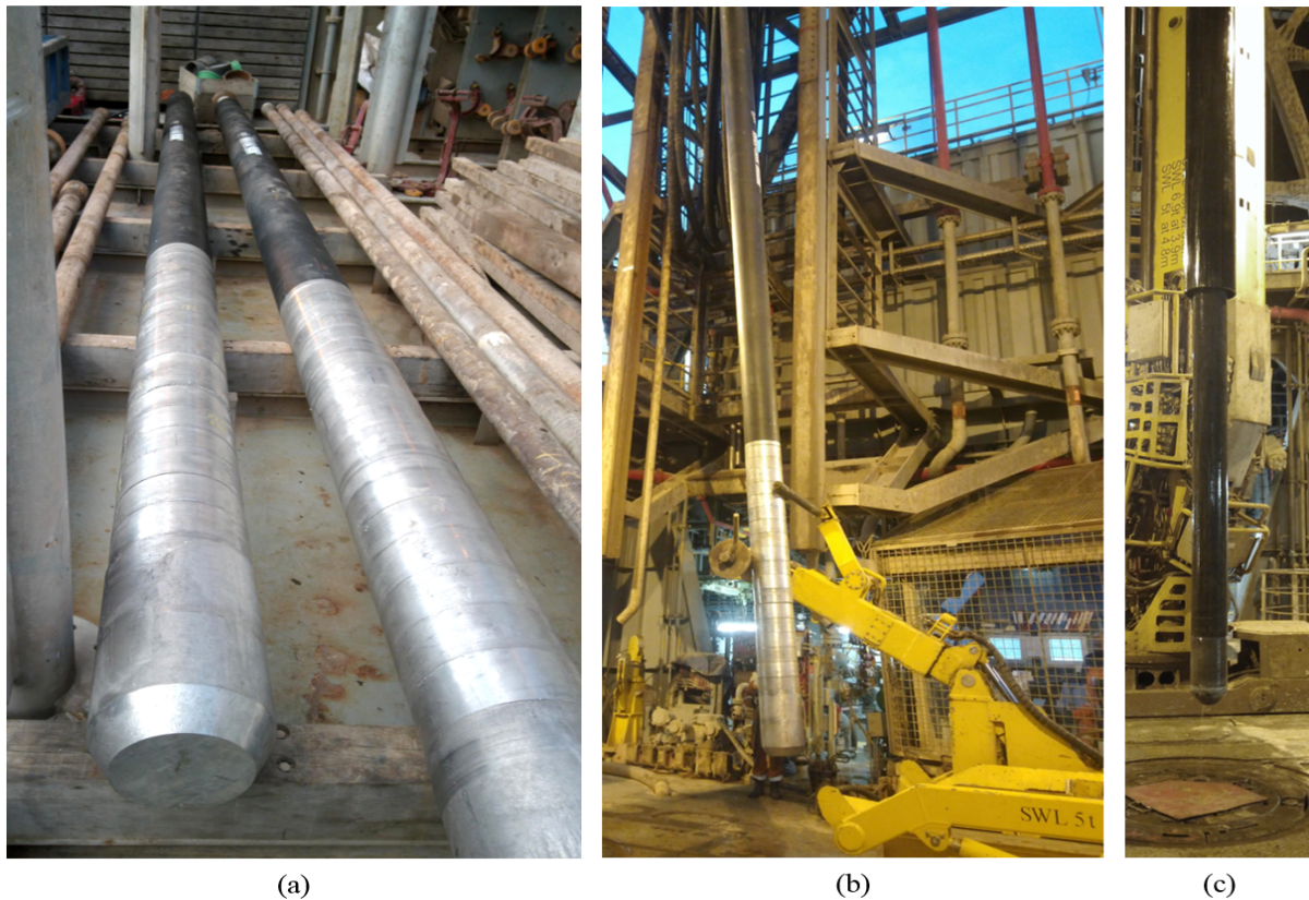
Figure 7.11: Bismuth plug assembly consisting of bismuth alloy and heater (a) Primary and back-up bismuth assembly. Heater sleeve is the upper black section. (b) Bismuth lifted in place and ready to be run in hole. (c) Thermite heater after melting bismuth. No bismuth alloy was observed on the heater.
