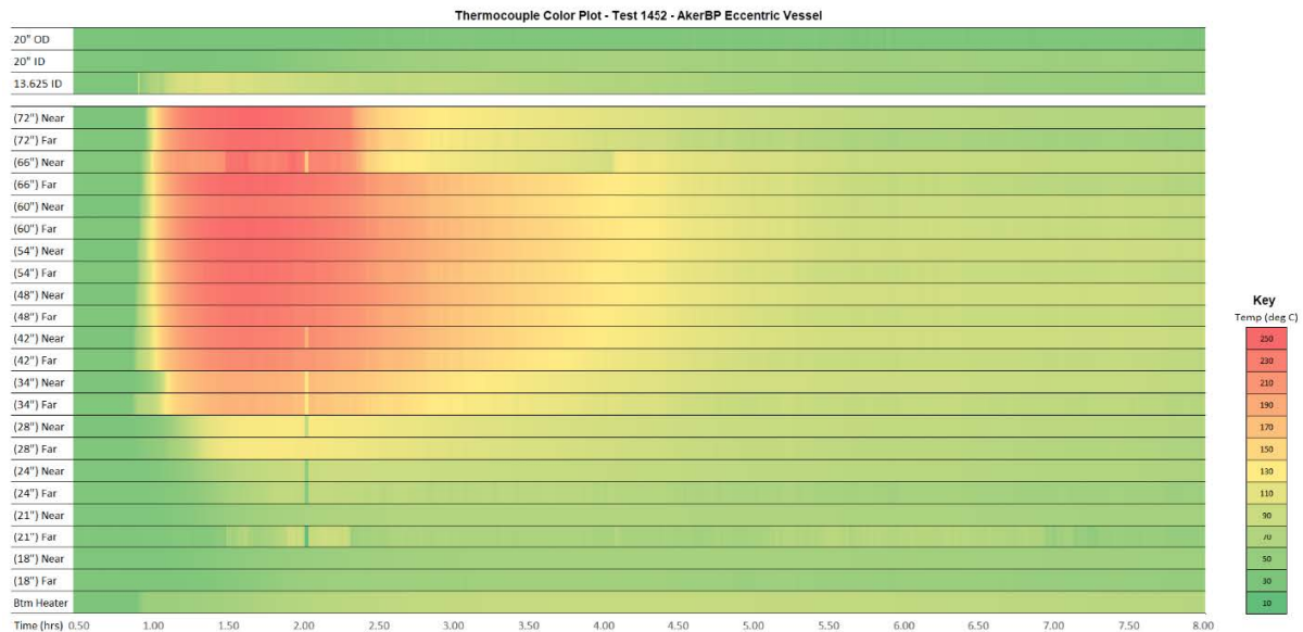
Figure 6.7: Temperature gradient during creation of a bismuth plug. Color plot are displaying temperature measurements over an 8 hour interval at different depths (distance from bottom in inches on the far/near side of the eccentric casing). Temperature decreases first in the top and bottom, causing the bismuth alloy to solidify here first. [Price and Elizondo, 2018]
