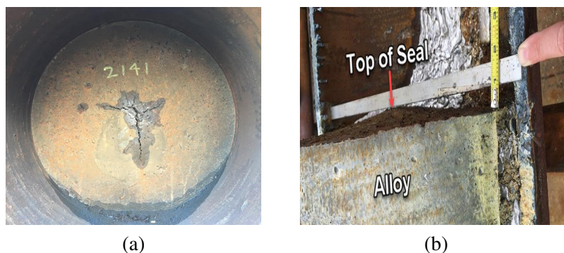
Figure 6.6: Inspection of the top of the final bismuth plug. (a) Top of the bismuth plug seen from above. (b) Demonstration of the top of the bismuth plug bulging out [Price and Elizondo, 2018]
