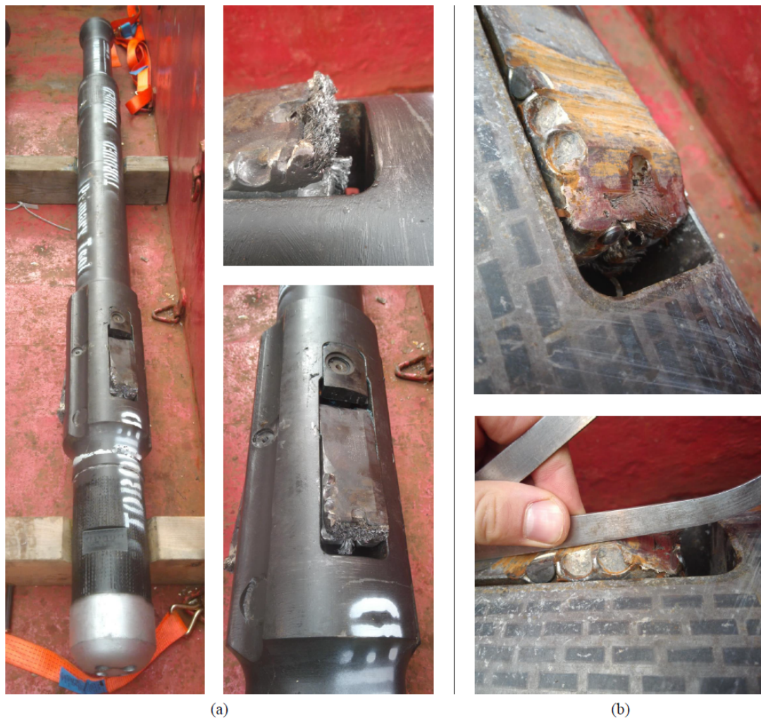
Figure 7.7: Special designed underreamer tool before and after. (a) Before run in hole. (b) After use.
