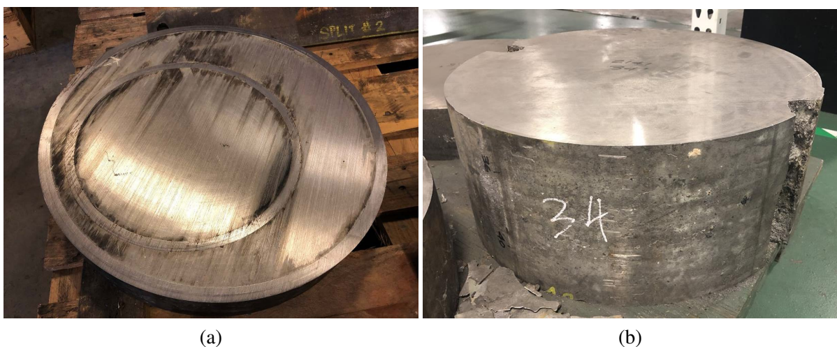
Figure 6.1: (a) Full cross section of plug when 13 3/8"x20" annulus is accessed by drilling holes in the 13 3/8" casing. (b) Saw cut section of final 20" bismuth plug deployed through a section milled interval in 13 3/8" casing (gouges along lengths are a result of torch cutting the 20" vessel open to retrieve plug). [Price and Elizondo, 2018]
