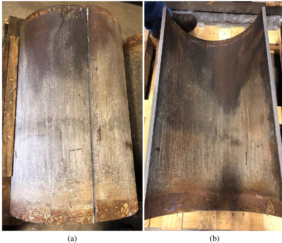
Figure 6.11: Silt lines observed during inspection of plug, representing potential leak paths along interface between alloy and casing. (a) Silt lines observed on outside of plug. (b) Silt lines observed on inside of casing. [Price and Elizondo, 2018]
