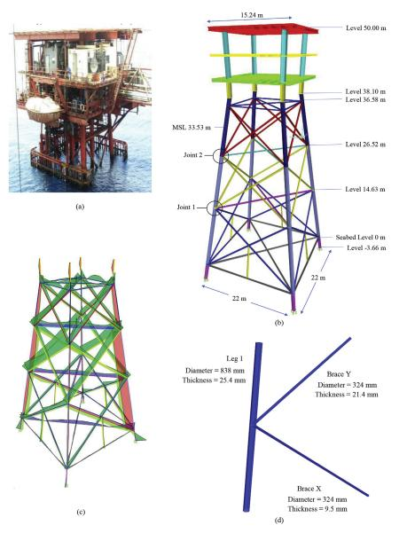
Fig. 3. (a) Considered offshore jacket platform (b) finite element model of the platform and critical joints (c) stress envelope in members for ULS assessment (d) details of critical joint 2.
