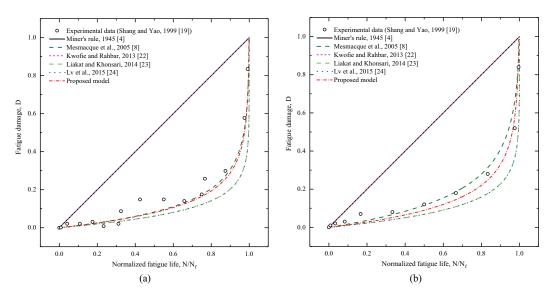
Fig. 2. Comparison of theoretically predicted fatigue damage evolution with experimental damage of 16 Mn steel for stress amplitude (a)  $\sigma_a$  = 337.1 MPa (b)  $\sigma_a$  = 373.5 MPa.
