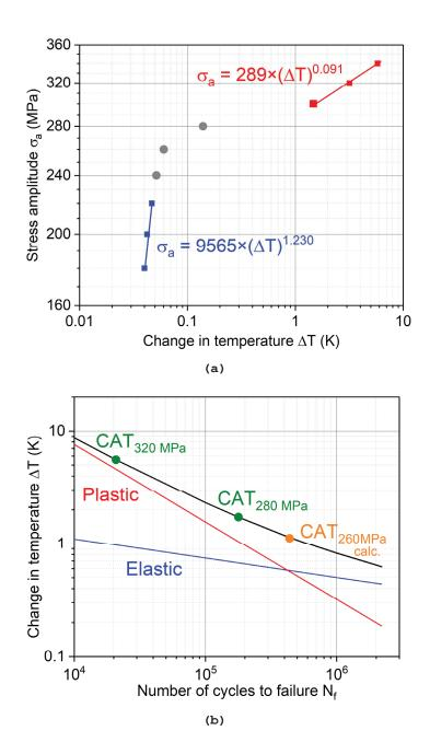
Figure 5. (a) Change in temperature with stress amplitude during LIT (b)  $\Delta T-N_f$  curve during CATs for S355 (SAE 1020) structural steel.
