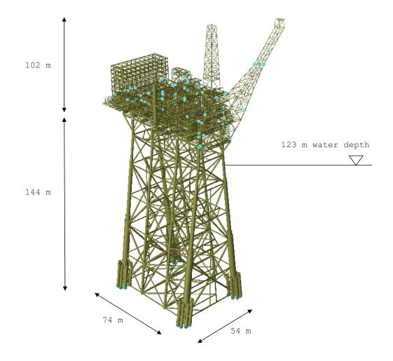
Figure 11. Finite element model of considered jacket type offshore structure and its dimensions.
