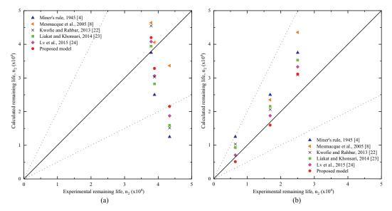
Fig. 5. Comparison of calculated fatigue life with experimental life for C 45 steel under (a) low-high loading (b) high-low loading.
