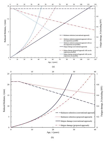
Fig. 4. Fatigue damage (including DFF) and member thickness variation with age in (a) critical joint 1 (b) critical joint 2.
