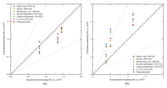
Fig. 7. Comparison of calculated fatigue life with experimental life for Al 2024-T42 under (a) low-high loading (b) high-low loading.
