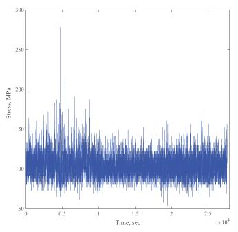
Figure 6. Considered variable amplitude loading for welded joints
