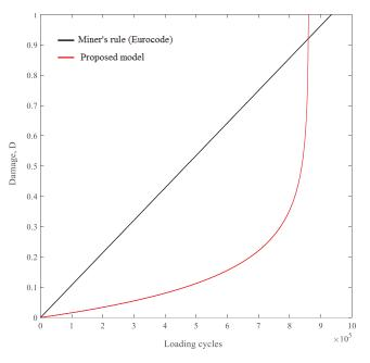
Figure 10. Fatigue damage accumulation using proposed model and Eurocode for butt welded joint
