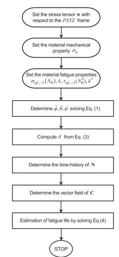
Fig. 1. Flowchart of the Carpinteri et al. criterion.
