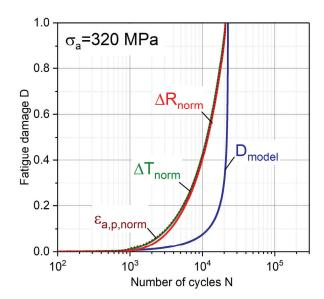
Figure 9. Comparison of experimental and calculated fatigue damage for CAT under  $\sigma_{a}$  = 320 MPa.
