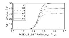
Fig. 3. S-curve shape, by varying the value of the parameter  $a\ (b=25$  and c=1.5).
