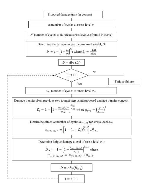
Figure 5 Flow chart of the proposed damage transfer concept [101]
