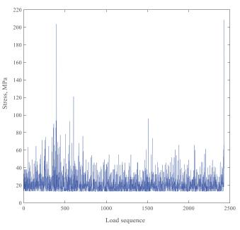
Figure 9. Stress history above endurance for fillet welded joint
