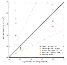
Fig. 13. Comparison of calculated fatigue life with experimental life for Al alloy under multilevel block loading.
