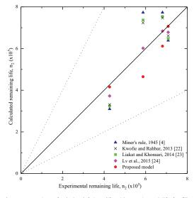
Fig. 18. Comparison of calculated fatigue life with experimental life for fillet welded joint.
