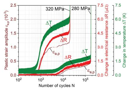
Figure 4. Constant amplitude test results for S355 (SAE 1020) structural steel.
