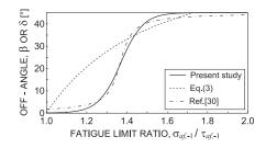
**Fig. 7.** Comparison between off-angle relationships: present study (Eq. (7) with a = 45, b = 18, and c = 1.37), original curve (Eq. (3)), and expression in Ref. [30].
