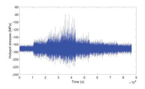
Figure 14. 24-hour time series for hot spot stresses in considered brace member.
