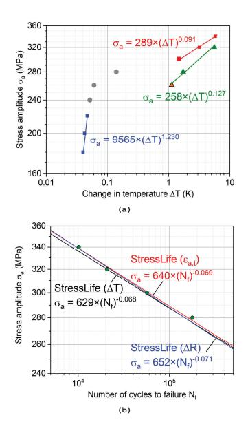
Figure 6. (a) Change in temperature with stress amplitude during LIT and CATs (b) comparison of the calculated StressLife<sub>tc</sub>-curves with conventionally determined S-N data of S355 (SAE 1020) structural steel.
