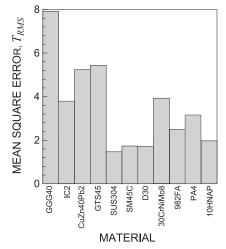
**Fig. 9.** Mean square error,  $T_{RMS}$ , by employing the original off-angle relationship (Eq. (3)).
