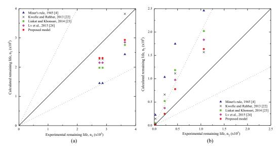
Fig. 10. Comparison of calculated fatigue life with experimental life for 30CrMnSiA under the loading (a) low high i.e.  $\sigma_1$  = 797,  $\sigma_2$  = 940 (b) high low i.e.  $\sigma_1$  = 940,  $\sigma_2$  = 797.
