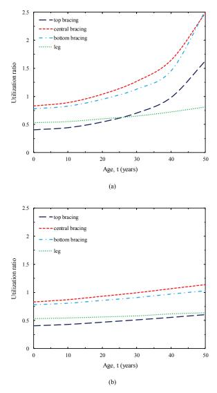
Fig. 7. Variation of ULS utilization ratio in critical members (a) conventional approach (b) proposed approach.
