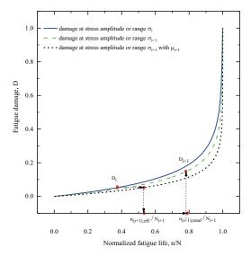
Fig. 3. Graphical representation of the proposed damage transfer concept.
