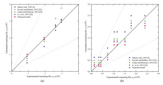
Fig. 11. Comparison of calculated fatigue life with experimental life for 30CrMnSiA under the loading (a) low high i.e.  $\sigma_1$  = 850,  $\sigma_2$  = 940 (b) high low i.e.  $\sigma_1$  = 940,  $\sigma_2$  = 850.
