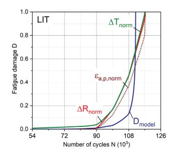
Figure 7. Comparison of experimental and calculated fatigue damage for LIT.
