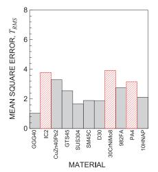
**Fig. 8.** Mean square error  $T_{RMS}$  by employing the novel off-angle relationship (Eq. (7) with a = 45, b = 18, c = 1.37). Results obtained from experimental data not used in the regression analysis are shown with diagonal hatching.
