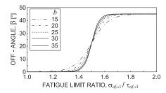
Fig. 4. S-curve shape by varying the value of the parameter b (a = 45 and c = 1.5).
