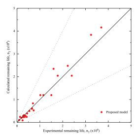
Fig. 8. Comparison of calculated fatigue life with experimental life for 30CrMnSiA under all loading sets.
