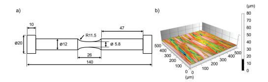
Figure 1(a) Specimen geometry for fatigue tests and (b) topography of polished specimen surface.
