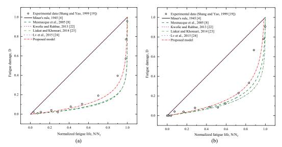
Fig. 1. Comparison of theoretically predicted fatigue damage evolution with experimental damage of C 45 steel for stress amplitude (a)  $\sigma_a$  = 330.9 MPa (b)  $\sigma_a$  = 405.8 MPa.
