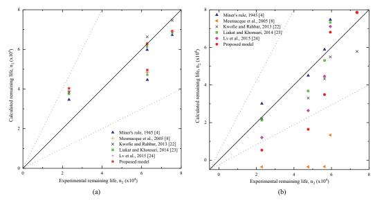
Fig. 6. Comparison of calculated fatigue life with experimental life for 16 Mn steel under (a) low-high loading (b) high-low loading.
