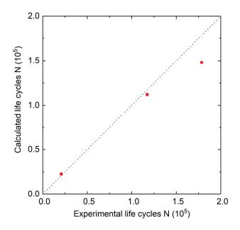
Figure 10. Experimental versus calculated life for fatigue life estimations under LIT and CATs.
