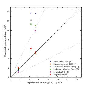
Fig. 12. Comparison of calculated fatigue life with experimental life for Al 6082-T6 under multilevel block loading.
