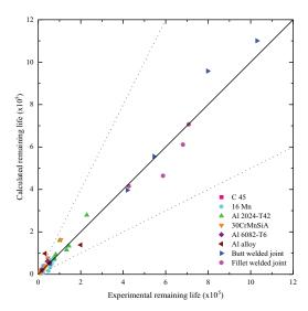
Fig. 19. Comparison of fatigue lives predicted by proposed model with experimental lives for all material and welded joints
