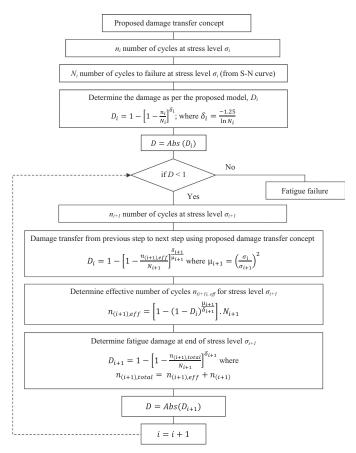
Fig. 4. Flow chart of the proposed damage transfer concept.
