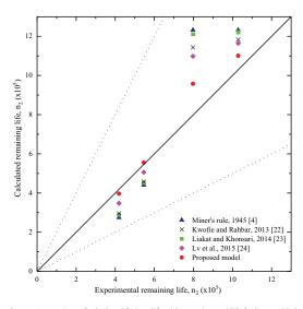
Fig. 17. Comparison of calculated fatigue life with experimental life for butt welded joint.
