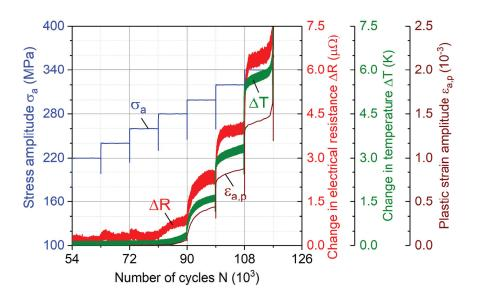
Figure 3. Load increase test results for S355 (SAE 1020) structural steel.
