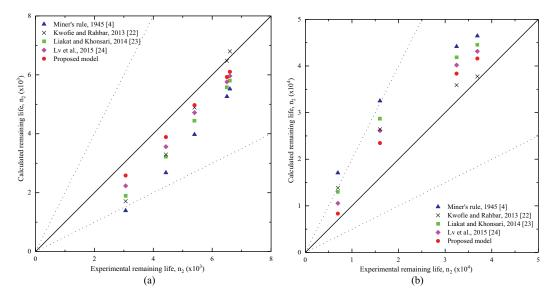
Fig. 9. Comparison of calculated fatigue life with experimental life for 30CrMnSiA under the loading (a) low high i.e.  $\sigma_1$  = 732,  $\sigma_2$  = 836 (b) high low i.e.  $\sigma_1$  = 836,  $\sigma_2$  = 732.
