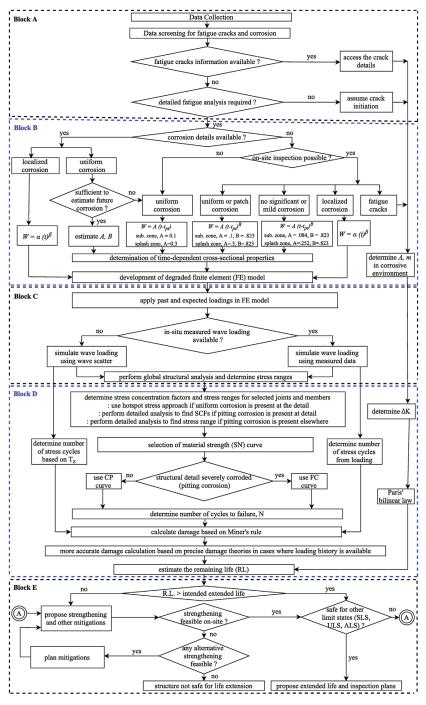
Fig. 1. Proposed framework for structural integrity assessment and life extension of ageing offshore structures.
