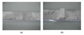
Fig. 14. (a) Butt welded joint test specimen (b) Fillet welded joint test specimen [41,42].
