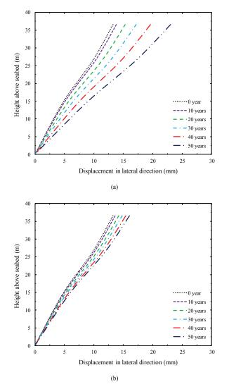
Fig. 6. Variation of leg displacement with age using (a) conventional approach (b) proposed approach.
