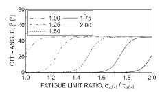
Fig. 5. S-curve shape by varying the value of the parameter c (a = 45 and b = 25).
