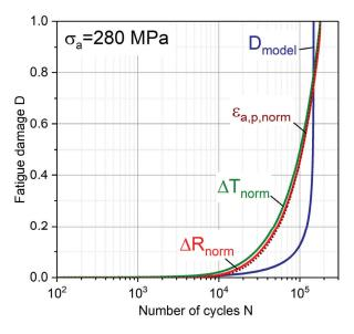
Figure 8. Comparison of experimental and calculated fatigue damage for CAT under  $\sigma_a$  = 280 MPa.
