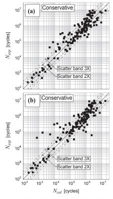
Fig. 10. Experimental fatigue life vs predicted fatigue life for each experimental data set analysed, by applying: (a) the novel relationship, (b) the original relationship. All results above the solid line  $N_{cal} = N_{exp}$  are conservative.
