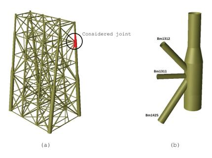
Figure 12.(a) Finite element model of jacket structure and considered
