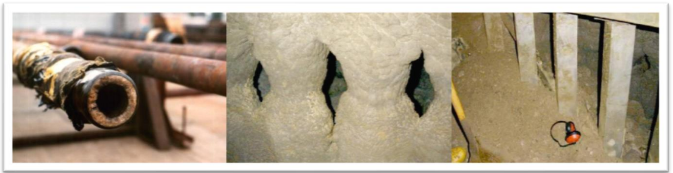
Figure 1. formation of scale a) in the pipeline, b) on separator surface and c) on clean separator surface. 3
