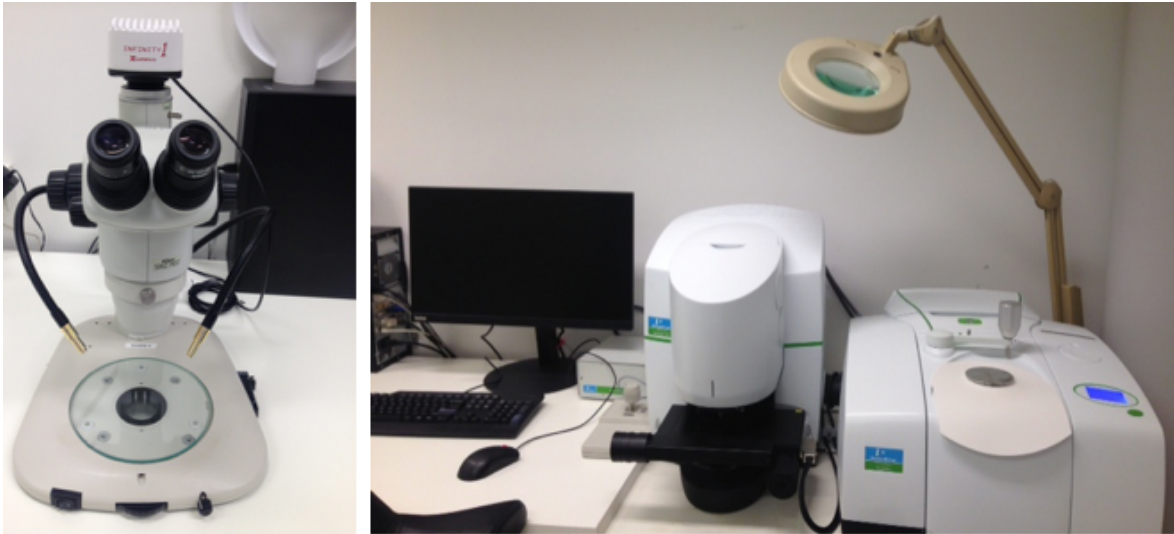
Figure 11. Microscope accoupled with the camera and the FT-IR.
