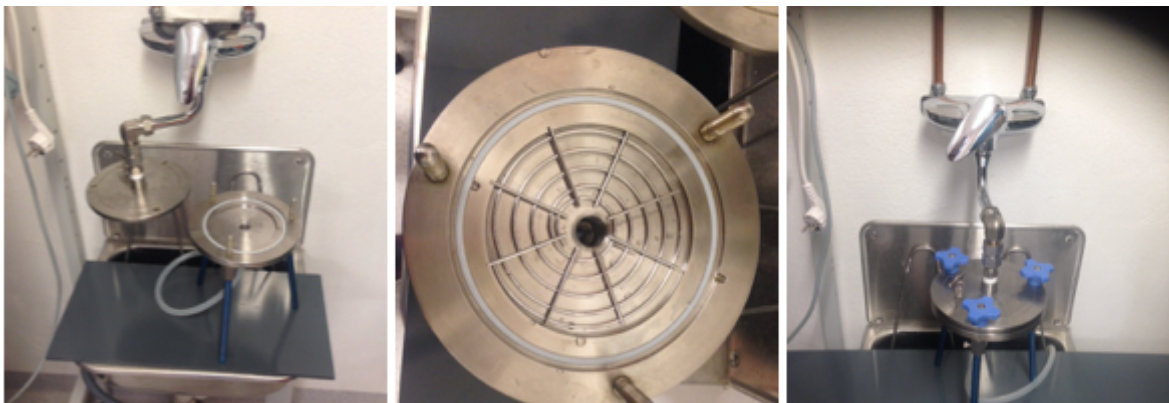
Figure 9. Filtration system for drinking water analysis samples.
