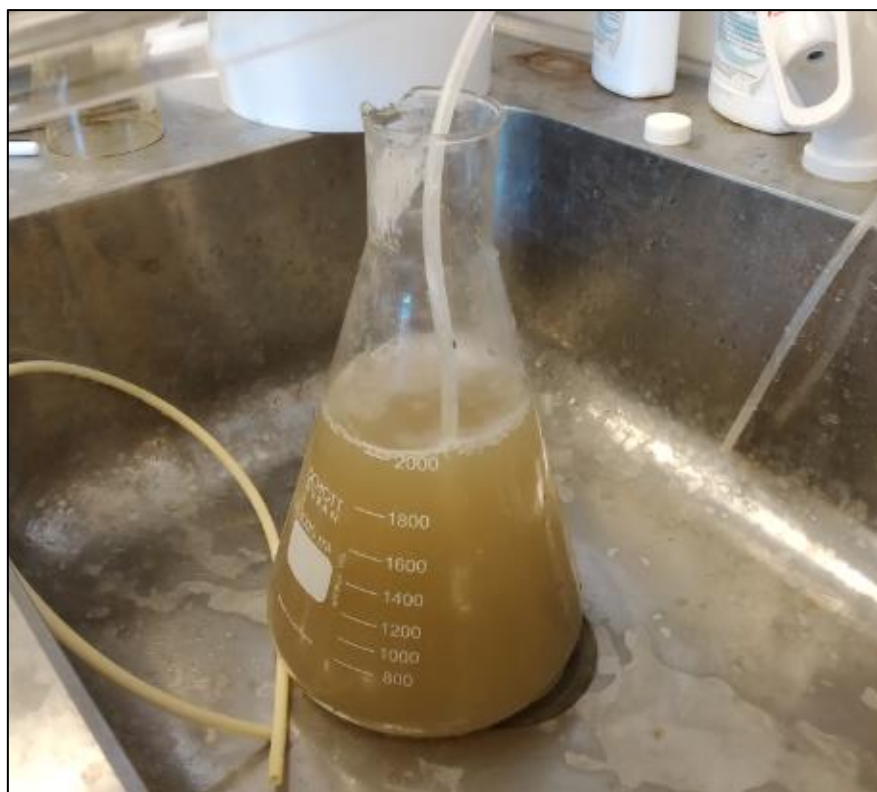
Figure 3.5: Simple SBR set-up
