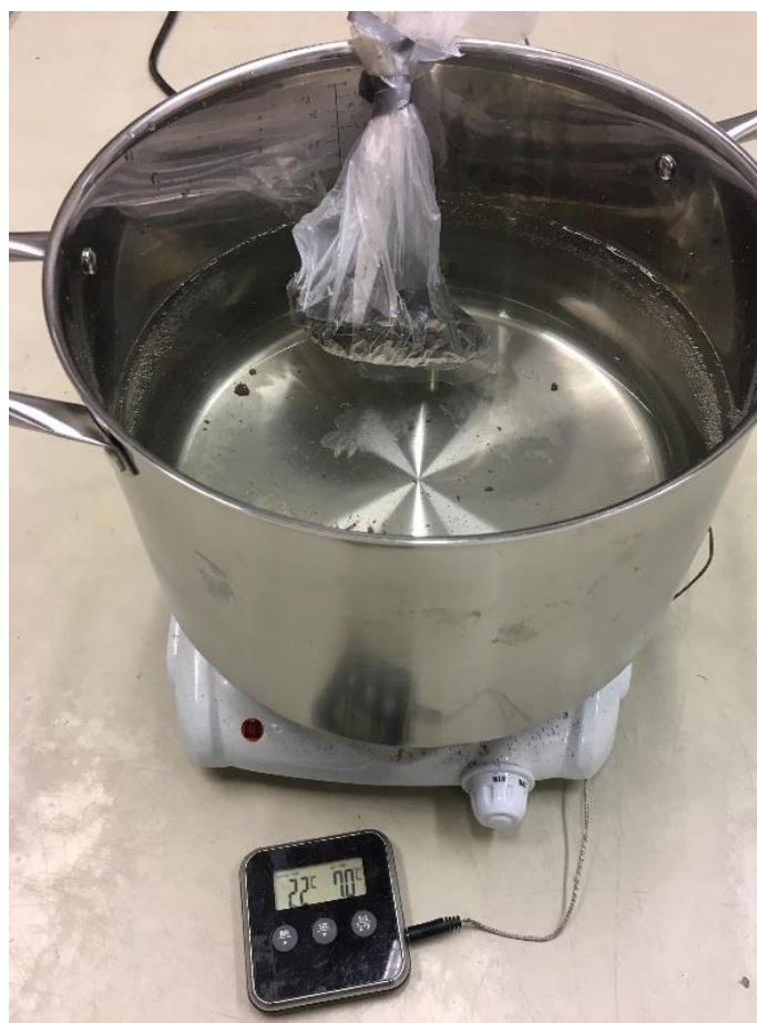
Figure 5-7: Set-up for heating of DC
