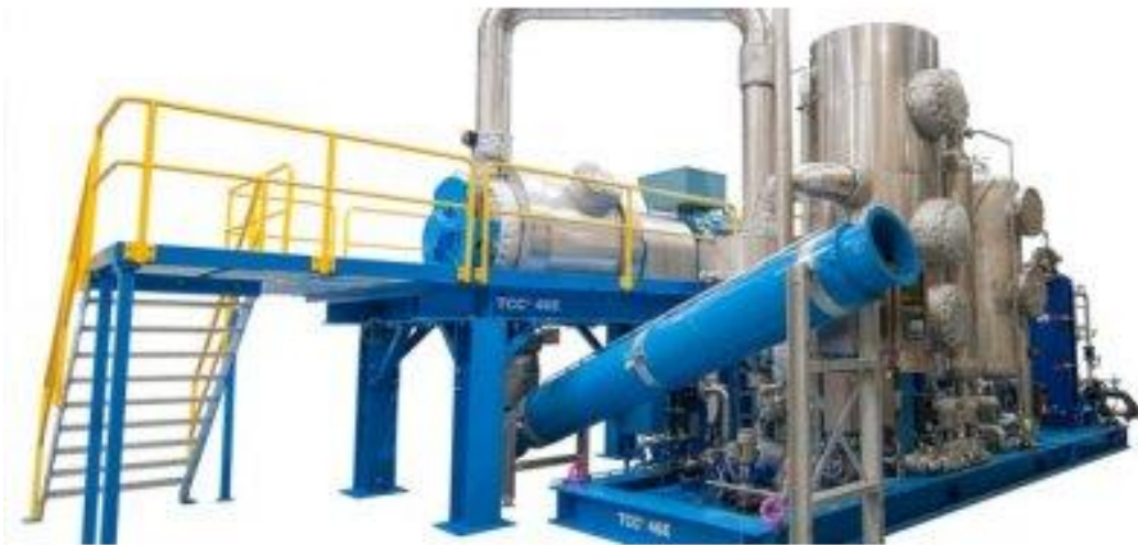
Figure 3-1: TCC unit (Thermtech AS, n.d.)
