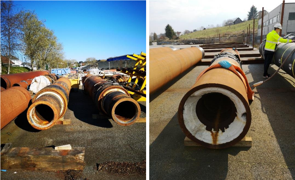
Figure 37 - Cut wellheads that will be used for testing
