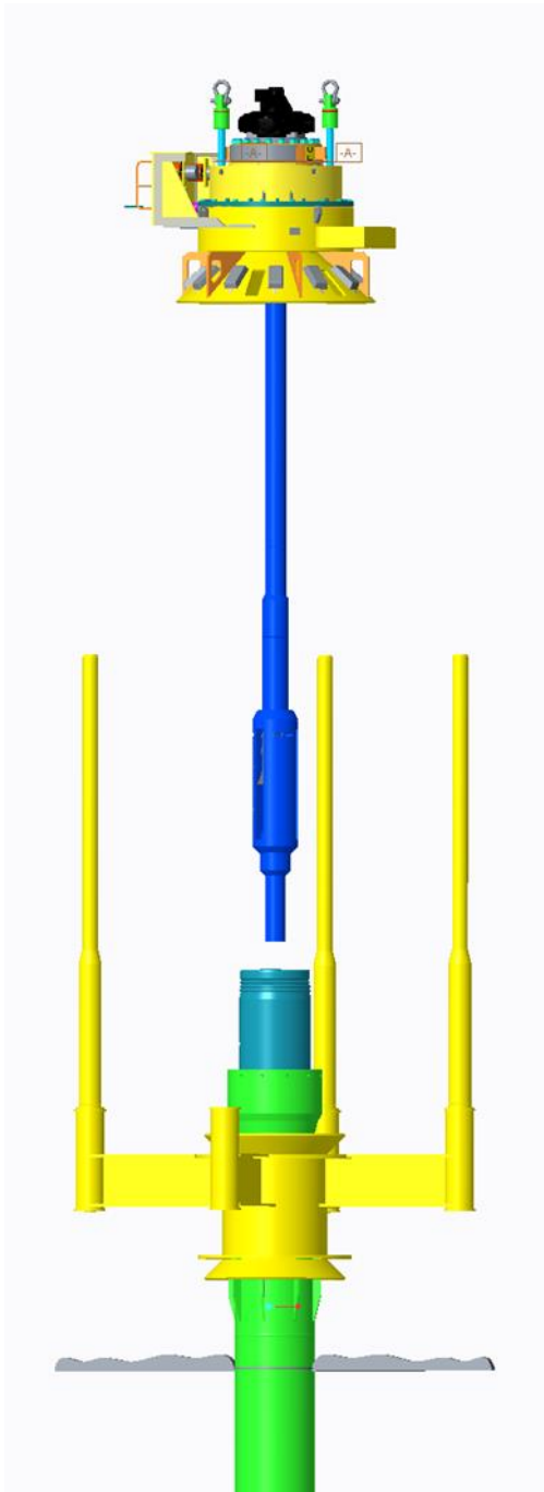
Figure 4 - Terminator entering a subsea wellhead with permanent guide base
