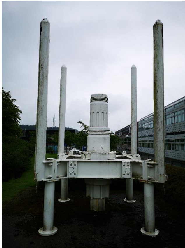
Figure 15 - Subsea wellhead with permanent guide base located on UIS campus
