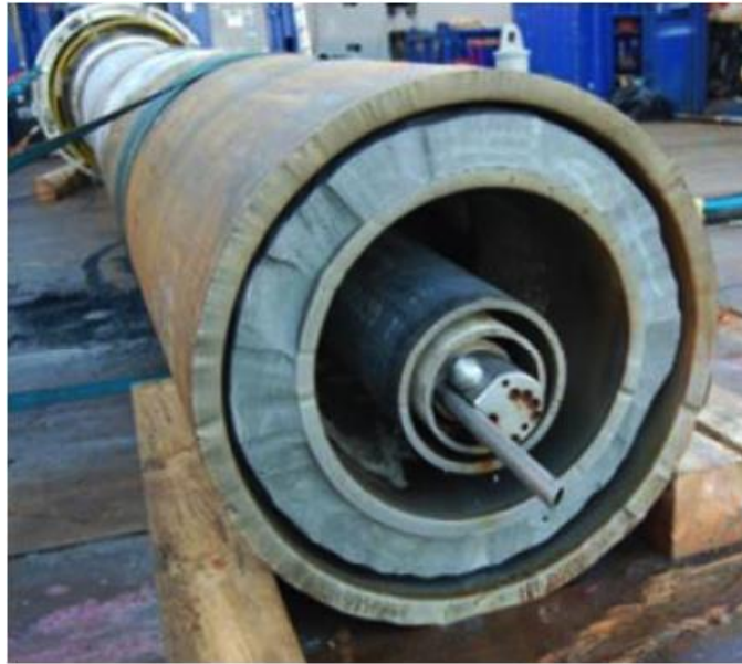
Figure 17 - Cut wellhead with AWJC tool still inside, from wellhead cutting campaign [83]
