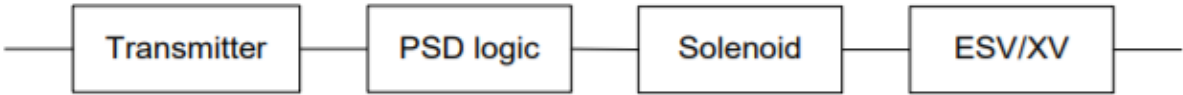
Figure 12 - ESD sub-system: Transmitter/sensor, logic solver and final element (solenoid, actuator and valve) [6, p. 78]
