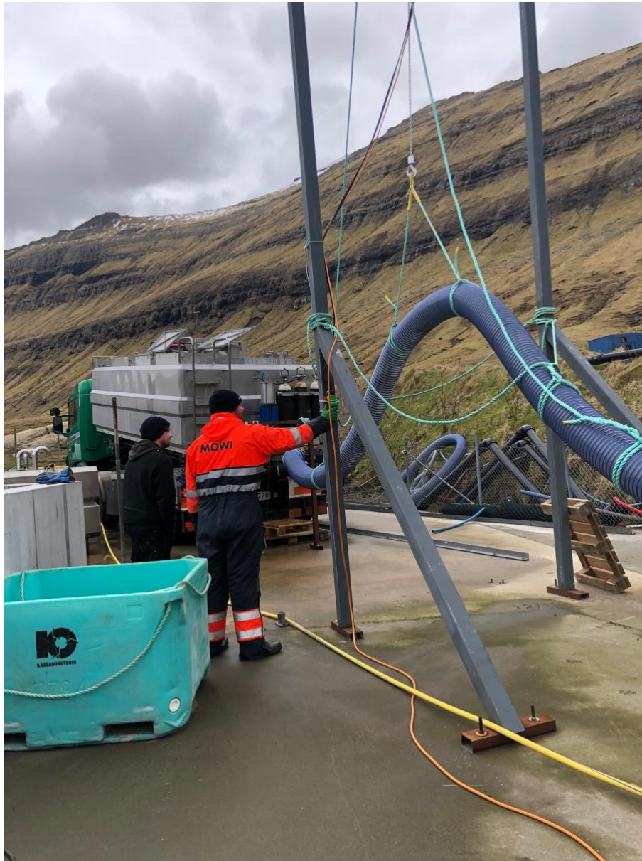
Figure 8: Transportation of fish from tanks through a pipe into the sea. Taken on a Mowi facility at the Faroe Islands 09.04.19.
