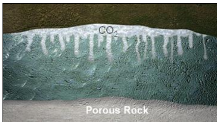
Figure 15. Solubility trapping, retrieved from https://www.co2captureproject.org/co2_trapping.html
