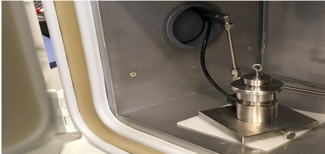
Figure_3.4 Small volume test kit with weight on top placed inside the thermal chamber
