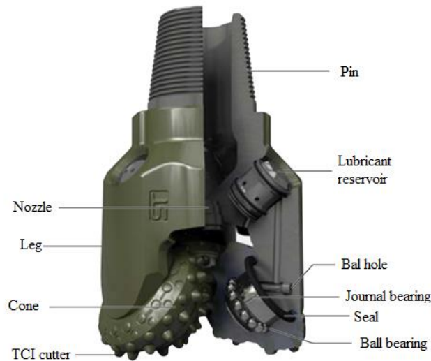
Figure 2.2 Major components of the Roller Cone Bit [7].
