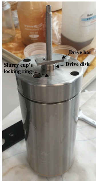
Fig. 3.6 The drive disk and the drive bar attached to the bottom of the slurry cup or the slurry cup's locking ring.
