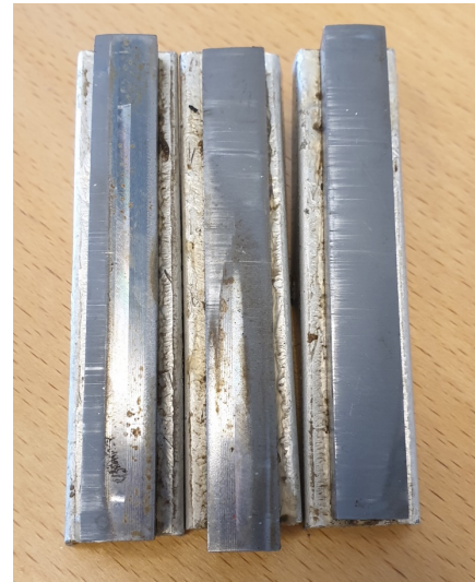
Fig. 3.8 A picture of the eroded surfaces of the three setup paddles after the experiments.
