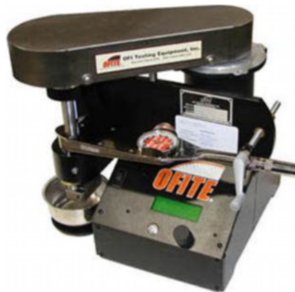
Fig. 1.5 EP and lubricity tester (after OFITE (2019a)).
