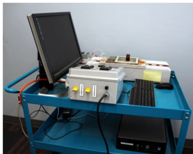
Fig. 1.6 Linear friction tester (after Livescu et al. (2014)).
