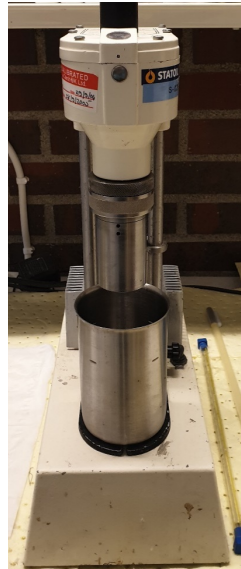
Fig. 4.16 Viscometer used for the rheology tests.
