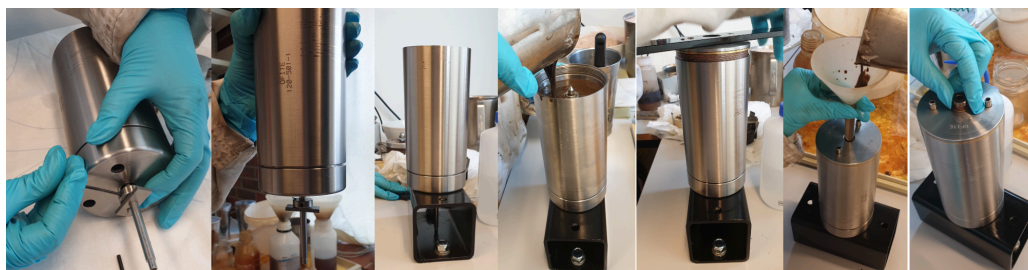
Fig. 3.3 The procedure of preparing the setup to be inserted into the HPHT consistometer.
