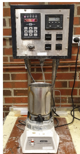
Fig. 2.5. The OFITE WARING commercial blender used for the mixtures prepared with the API mixing procedure.
