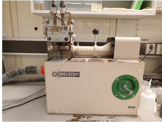
Fig. 2.8. The cutting machine used for cutting and flattening the ends of the samples for the UCS and the tensile strength tests.
