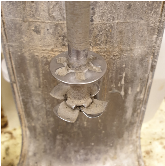
Fig. 2.2. The blades of the Hamilton Beach mud mixer used for mixtures prepared with the non-API mixing procedure.
