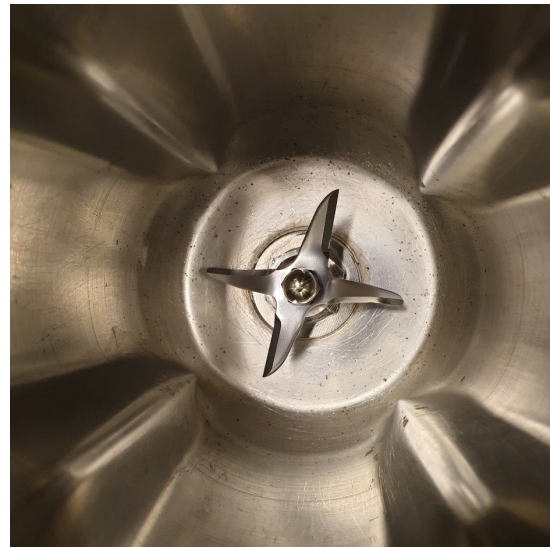
Fig. 2.3. The blades of the OFITE WARING commercial blender used for mixtures prepared with the API mixing procedure.
