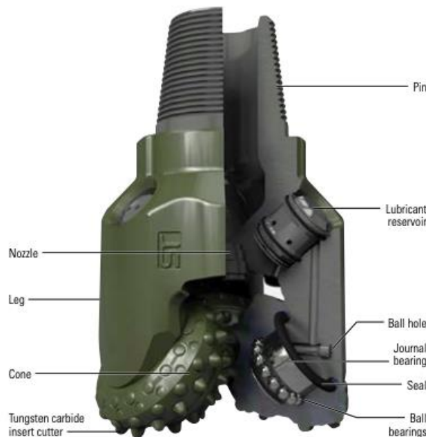
Figure 2. Roller Cone bit and its components [13].
