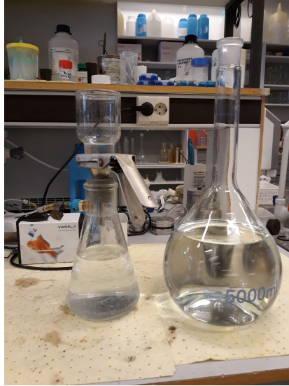
Figure 15: Filtration set-up showing the Vacuum Pump(Left) Filter(Middle) and Stock solution (right)
