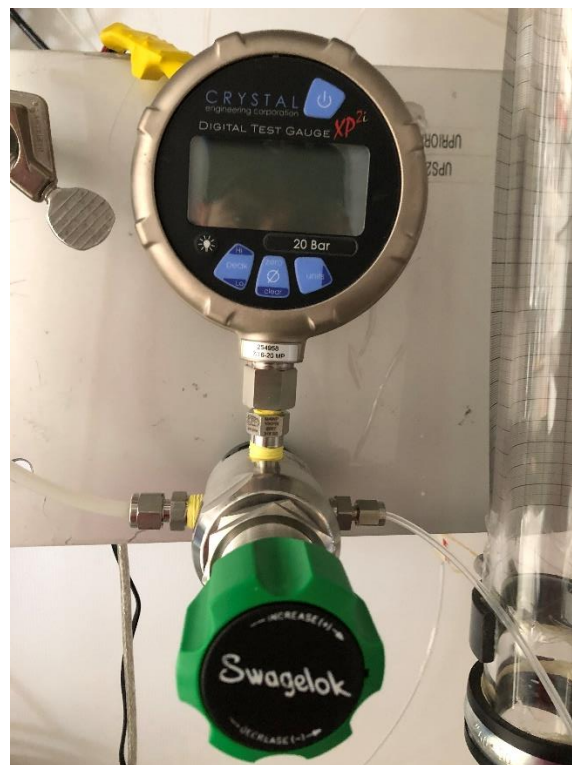
Picture 73. Swagelok pressure regulator and crystal engineering xp2i digital pressure gauge indicator
