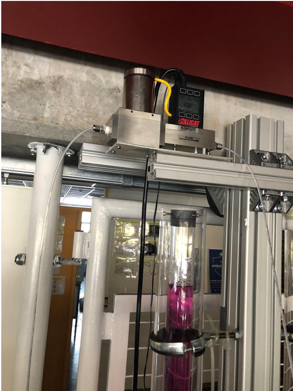
Picture 76. Air flowmeter.
