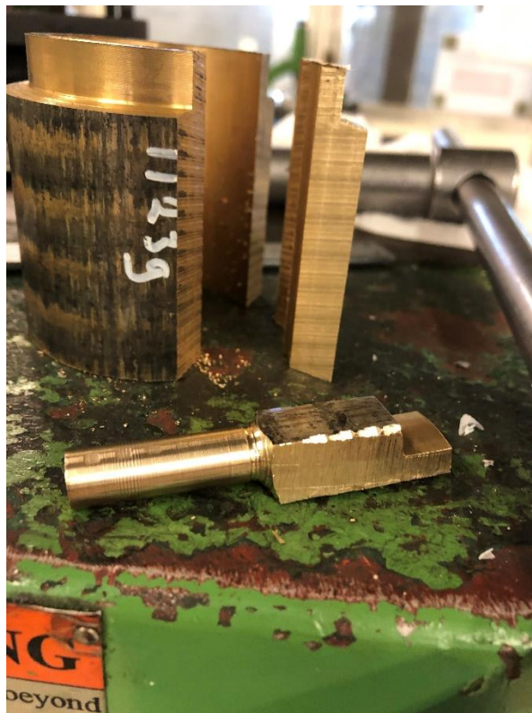
Picture 37. Temperature sensor holder during construction.
