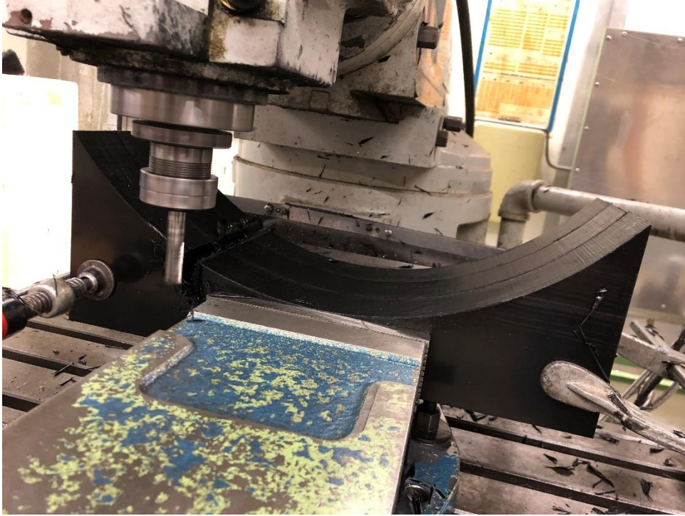
Picture 54. Separator support (cushions).
