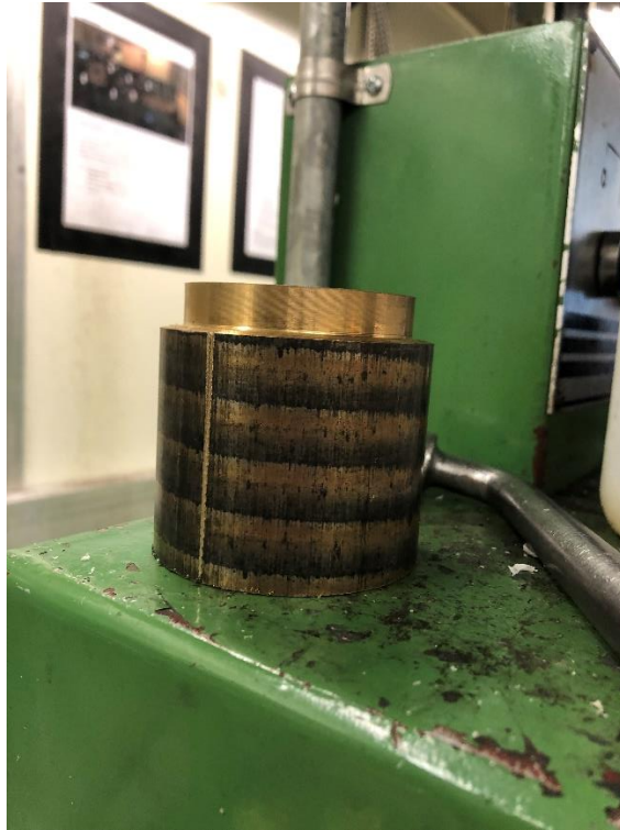
Picture 36. Temperature sensor holder during construction.
