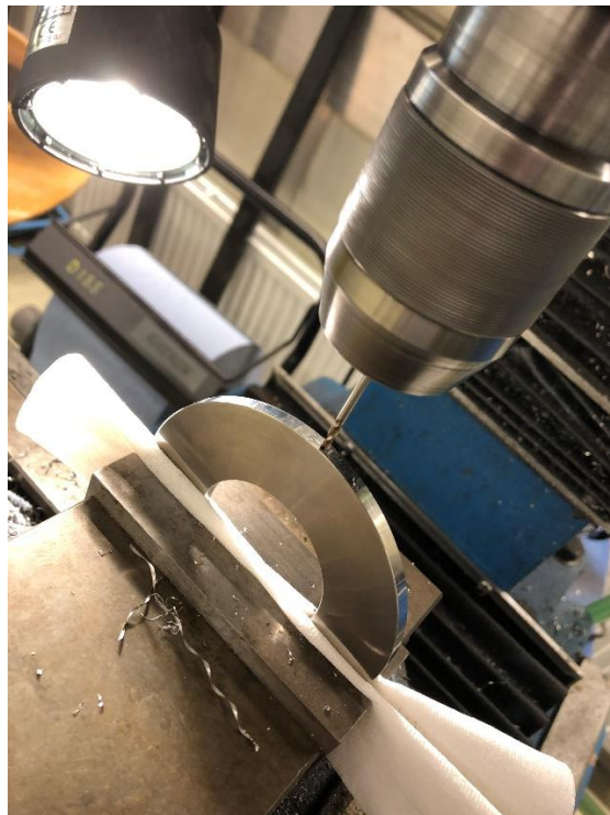
Picture 12. Earthing rings.
