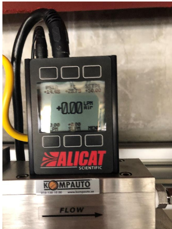
Picture 75. Air flowmeter
