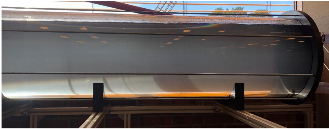
Figure 5.8. water level higher than the inlet.
