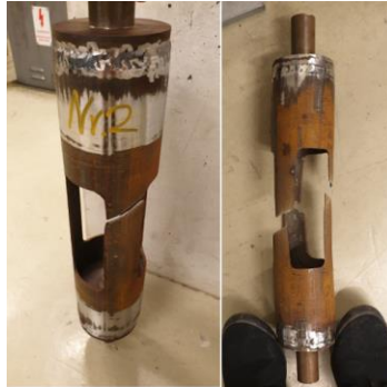
Figure 46 Tensile test of 89,1 mm x 3,0 mm
