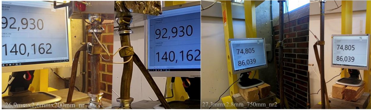
Figure 54 Capture from video; 27,3 mm x 2,8 mm graph comparison of smallest to longest unsupported lengths
