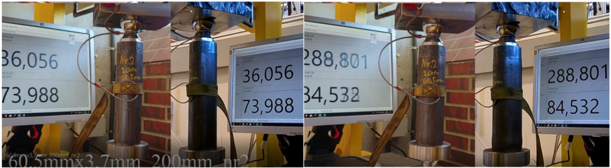
Figure 4 Video capture of strain hardening of 60,5 mm pipe with 332 mm unsupported length
