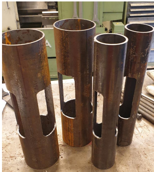
Figure 35 Pipe prepared for tensile test with cut out area for reduction of steel strength
