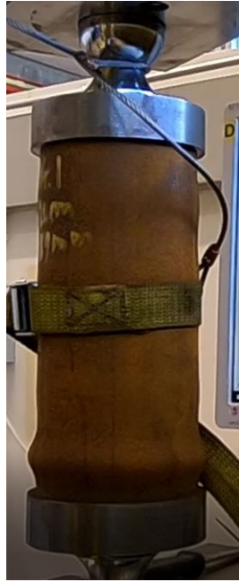
Figure 86, 89,1 mm x 3,9 mm, 332 mm unsupported length, short column compression failure
