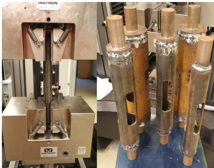
Figure 36 Tensile test machine and prepared pipes for testing
