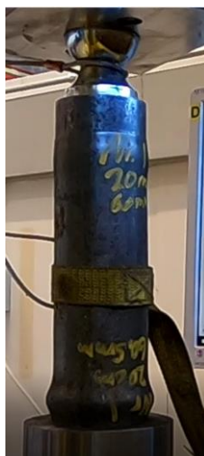
Figure 72 Deformation of tubing during compression testing
