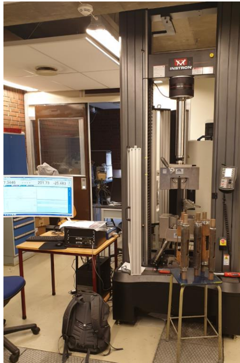
Figure 29 Instron 5985 dual column floor frames tensile test machine
