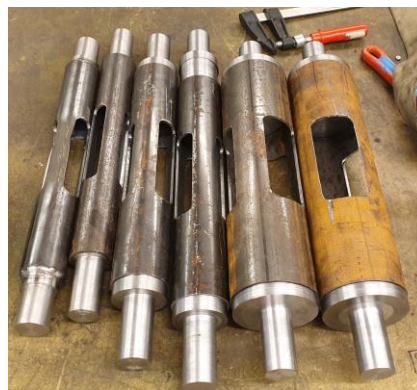
Figure 31 Prepared bushing ready to be welded
