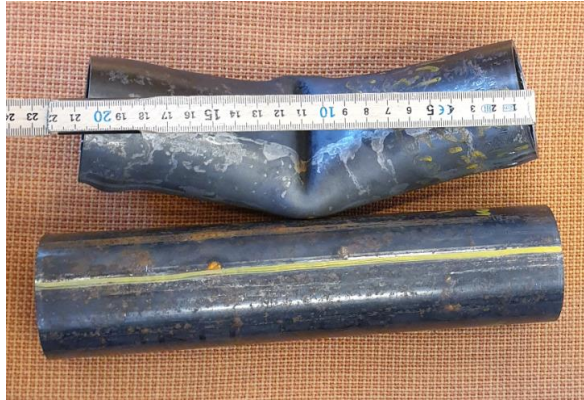
Figure 59 Picture of 33,9mm x 3,2mm pipe after the compression test
