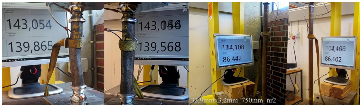
Figure 61 Capture from video; 33,9 mm x 3,2 mm graph comparison of smallest to longest unsupported lengths
