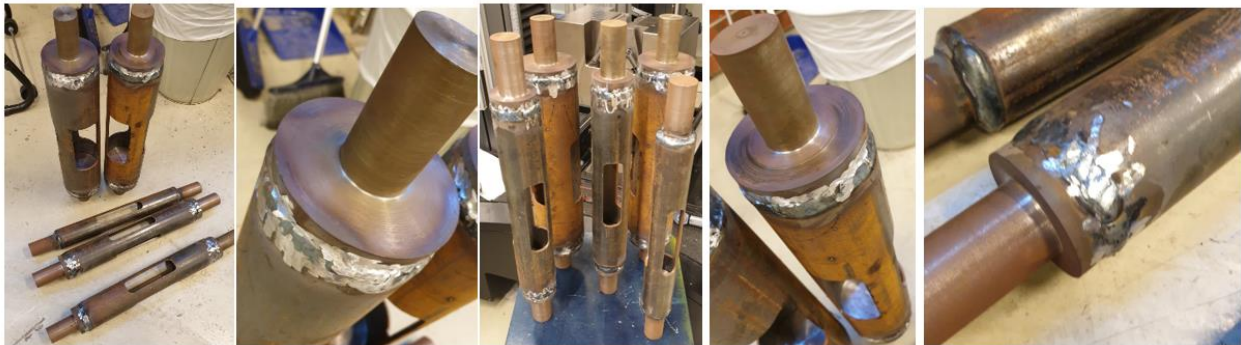
Figure 25 Welded bushing to pipes
