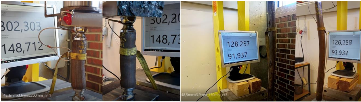
Figure 67 Capture from video; 48,5 mm x 3,9 mm graph comparison of smallest to longest unsupported lengths
