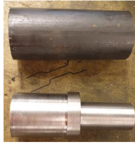
Figure 23 Bushing for tensile test example
