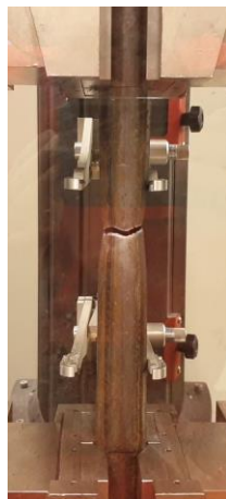
Figure 38 Tensile test picture of 27,3 mm x 2,8 mm pipe
