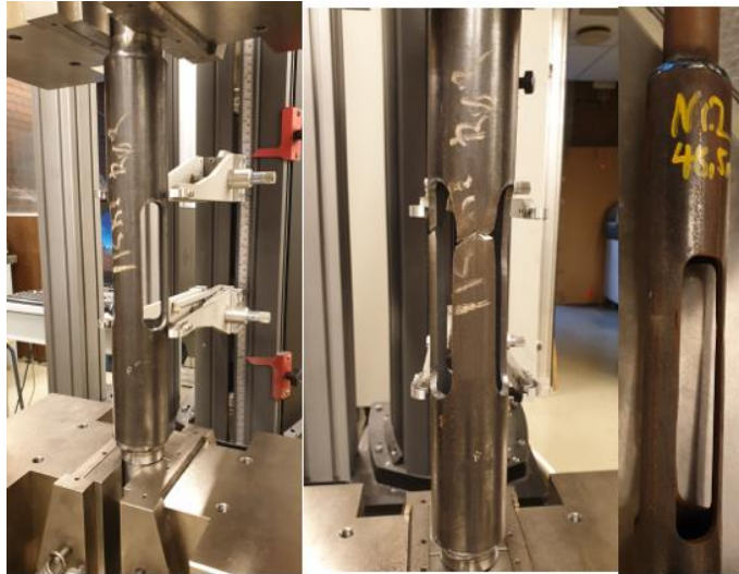
Figure 42 Tensile test picture of 48,5 mm x 3,9 mm pipe
