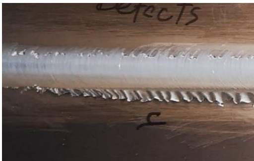
c) Wormhole and lack of filling
