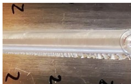
d) Weld at last 50 mm having some flash
