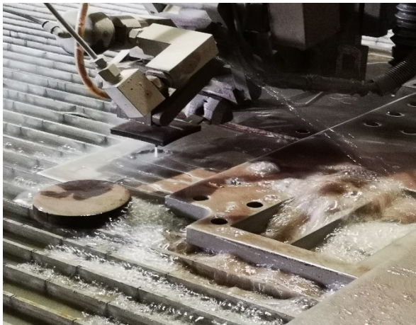
a) Waterjet cutting in progress
