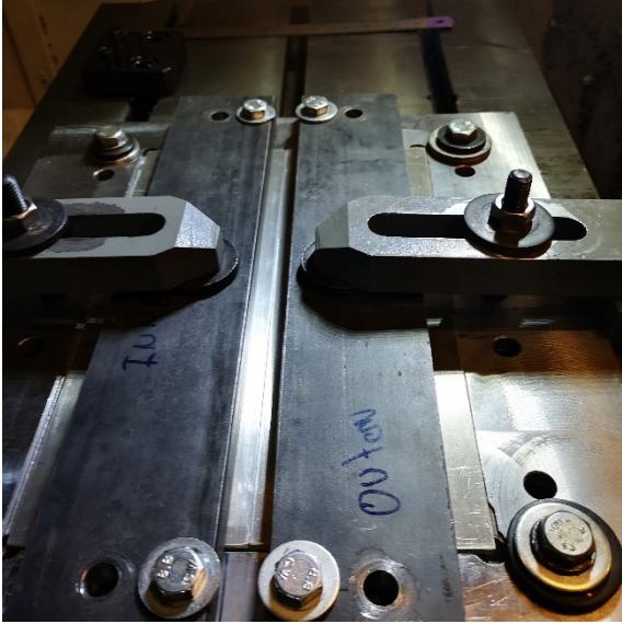
b) Ready to be welded plates
