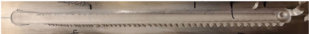
a) Frontside of Experiment 4, wormholes, lack of filling and flash.
