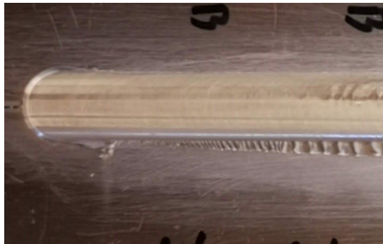
c) Start of the weld with low shoulder
