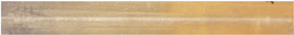
b) Backside of weld showing good quality
