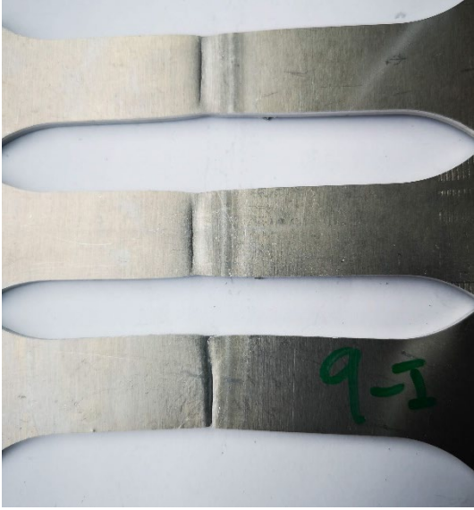
g) Backside after Tensile Testing from below
