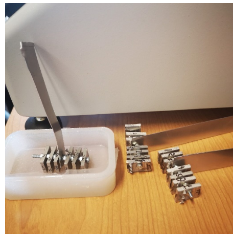
f) Inside the mould ready for epoxy
