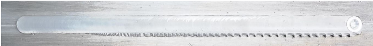
a) Frontside of Optimum Weld advancing side at the top. Flash at retracting side
