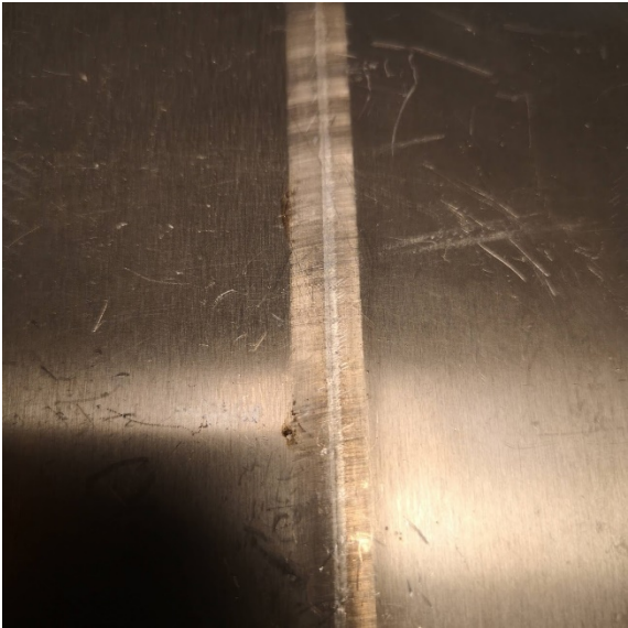
b) Backside of weld
