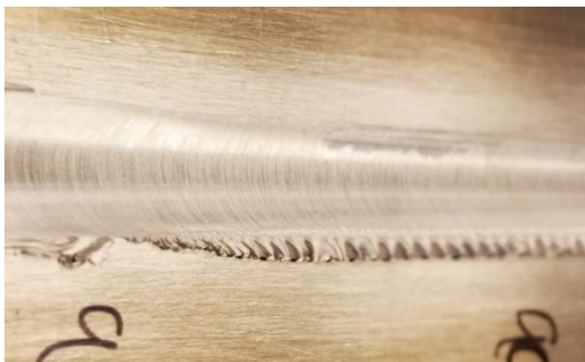
c) Irregular Surface and flash
