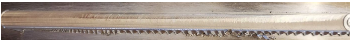
a) Frontside of weld with visible flash at retracting side
