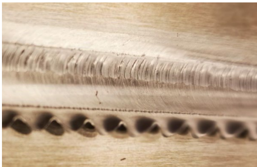
c) Irregular Surface and flash
