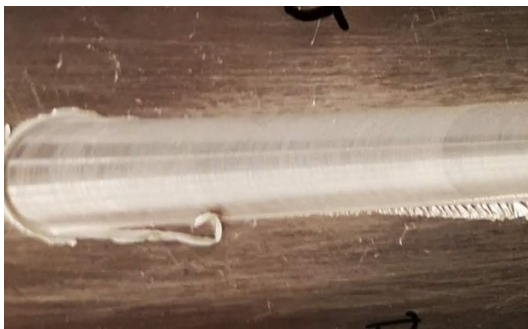
c) Start of the weld with low shoulder depth
