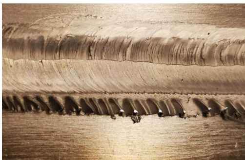
c) Irregular surface and excess flash RS.
