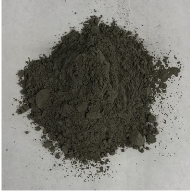
Binder CEM II/A-V 42,5 N (Norcem Anleggsement FA) Density: 3020 \text{ kg/m}^3 Blain: 390 \text{ m}^2/\text{kg}
