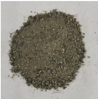
Aggregate Gneiss-granite Particle diameter 0-4mm Density: 2660 \text{ kg/m}^3
