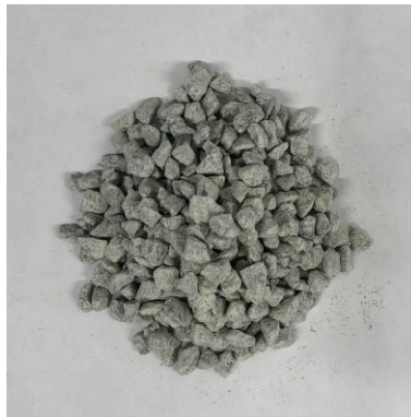
Aggregate Quartz-diorite Particle diameter 5-8mm Density: 2770 \text{ kg/m}^3
