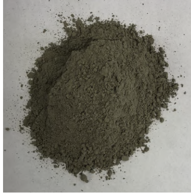
Binder CEM I 52,5 R (Norcem Industrisement) Density: 3130 \text{ kg/m}^3 Blaine: 550 \text{ m}^2/\text{kg}
