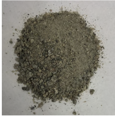
Aggregate Hostrup quartz sand Particle diameter 0-1mm Density: 2640 \text{ kg/m}^3
