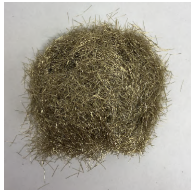
Steel fiber (Weidacon) Length: 9 mm Diameter: 0.15 mm Aspect ratio: 60
