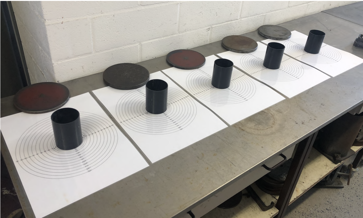
Figure 3.1: Miniature slump flow to measure workability over time
