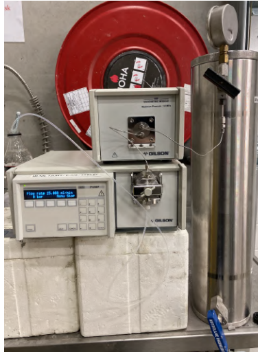
Figure 5.14: Pressure tank used to determine the pressure saturated porosity.
