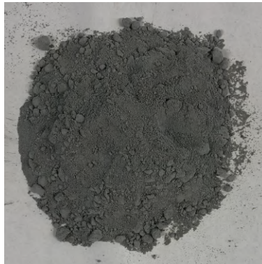
Binder Silica fume (Elkem microsilika 940U) Density: 2650 \text{ kg/m}^3
